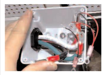
Of all the factors that affect the efficiency of a bilge pump's operation, wire size or gauge is perhaps the most important. Undersized wires can seriously diminish a pump's capacity while giving no outward sign of a problem. Ideally, bilge pump wiring should present *no more* than a 3 percent voltage drop.
