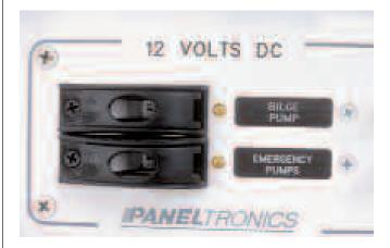
It's important that bilge pumps be installed in such a way that they cannot be inadvertently shut off. Having a protected or covered circuit breaker is one option, or a fuse can be used. The latter choice is not as convenient to service and requires that spares be kept on hand.
