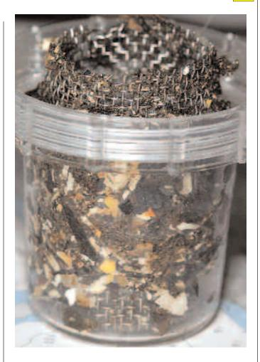
Debris is a bilge pump's worst enemy. This strainer, installed aboard a new vessel, has become impacted with "new-build debris," rendering the bilge pump it serves useless. The watch phrase for pump-savvy cruisers is: keep your bilges clean and free of all debris, no matter how small or seemingly insignificant.
