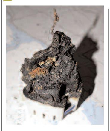
Bilge pump electrical components—float switches, manual switches, wiring, and so forth—must be capable of handling the loads imparted on them by the bilge pump under all operating conditions. This float switch was not defective; it was simply underrated for the pump's ampere draw.
