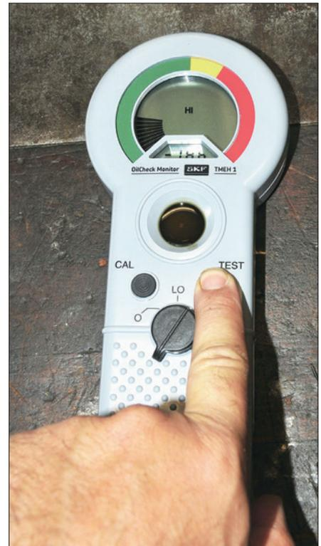
This field oil-analysis tool is particularly useful in remote locations where sending in samples for testing is impossible. While it can't match the capabilities of a full laboratory, the tool can comparatively assess used crankcase oil relative to a sample of the same variety of new oil. **Left**—The sensor pad is washed with solvent prior to a test. **Right**—A sample of used oil on the sensor pad is tested.
