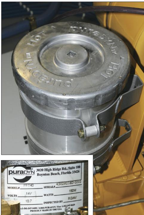
**Left**—Not factory original, this bypass filter system, like most, was added after the engine was purchased and installed in a boat. It requires little maintenance save filter replacement, and has serviced thousands of gallons of oil over the years. **Right**—This puraDYN bypass filtration system is fitted with an electrical heating element to promote evaporation of water from oil that regularly circulates at less-than-optimum operating temperature.
