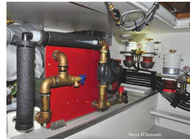
Left: The engineering space under the saloon sole is bright, neatly laid out, and accessible, making service for the primary fuel filters and polishing system hassle free. Right: The Coastal Craft 56 is equipped with a state-of-the-art Kabola diesel furnace that includes in-sole radiant heating.
