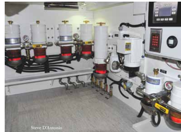
Left: The engineering space under the saloon sole is bright, neatly laid out, and accessible, making service for the primary fuel filters and polishing system hassle free. Right: The Coastal Craft 56 is equipped with a state-of-the-art Kabola diesel furnace that includes in-sole radiant heating.
