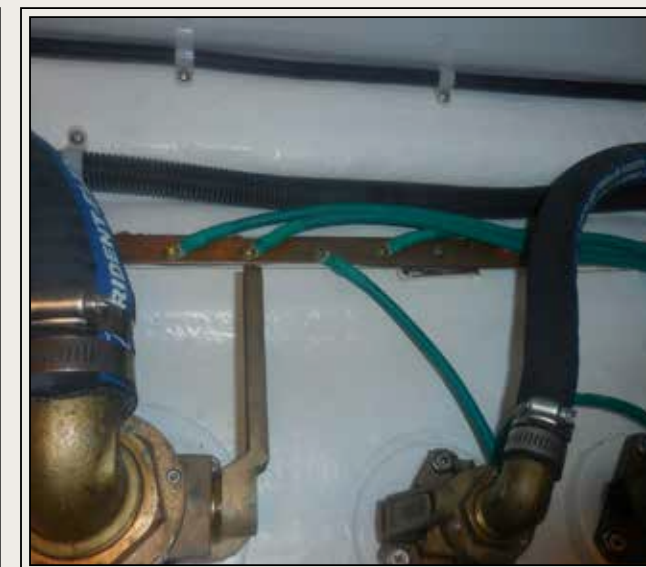
The bonding system, typically wired using green (sometimes with a yellow stripe) insulation, relies on good, clean, low-resistance connections. Ideally, heat-shrink terminals, or supplemental heat-shrink tubing should be used, and connections should be coated with a corrosion inhibitor. Each piece of underwater metal requires a bonding wire (right).
