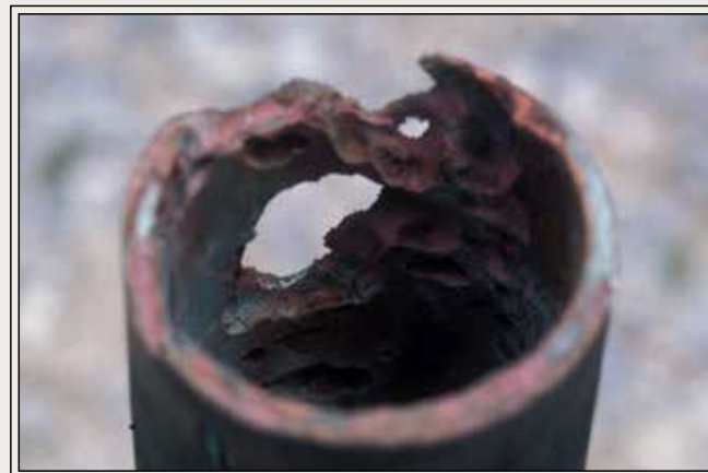
Galvanic isolators are used to protect boats that are berthed in proximity of each other from damage when they're plugged into shore power (above, left). An aluminum bracket is being eaten away as water drips on it from a bronze pump (top, right). A metal shaft log corroded because the alloy it was made of contained too much zinc.
