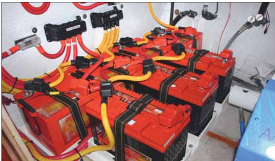
Left —All batteries (even the sealed type) that are stored aboard will require maintenance. Above —Battery banks and monitoring systems on deep-stored boats should be periodically inspected by a knowledgeable electrician. He or she should visually check connections, case condition, and voltage, and monitor temperatures while charging.
