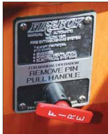
Left —Whenever possible, manual discharge handles should be installed in plain view. If one is placed in a locker, clearly label it to indicate its presence. Center —The exposed manual discharge handle is missing its arming pin. Right —Be certain you and your customer understand that the indicator light goes out once the system has discharged.
