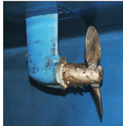
Left —An alternative to a conventional propeller, shaft, and strut is to attach the wing engine to a sail drive for get-home service. Relatively easy to install through a single hole in the hull bottom, the sail-drive system presents a streamlined underwater profile and is fitted with a proprietary folding prop ( above ).
