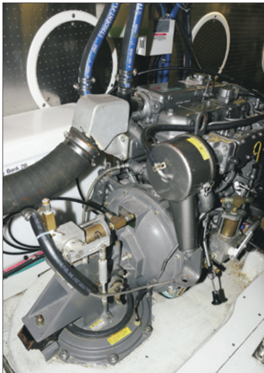
Left —An alternative to a conventional propeller, shaft, and strut is to attach the wing engine to a sail drive for get-home service. Relatively easy to install through a single hole in the hull bottom, the sail-drive system presents a streamlined underwater profile and is fitted with a proprietary folding prop ( above ).
