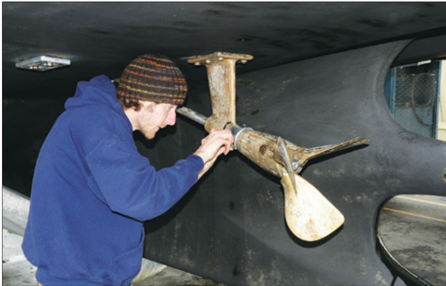
Above —During a haulout the running gear for the wing engine should be given the same attention as the main prop and shaft, including cursory inspection of shaft alignment and Cutless bearings, and replacement of anodes. Left —The gear mechanisms of folding props should be cleared of any marine growth and packed with grease to ensure that they function reliably.
