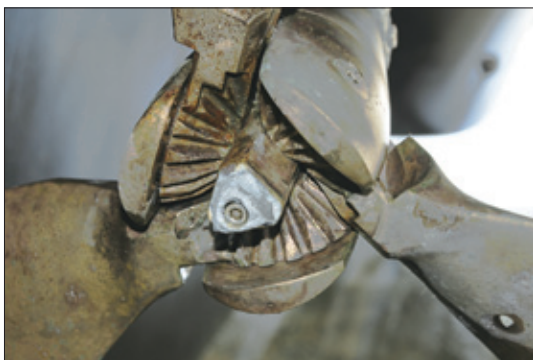
Above —During a haulout the running gear for the wing engine should be given the same attention as the main prop and shaft, including cursory inspection of shaft alignment and Cutless bearings, and replacement of anodes. Left —The gear mechanisms of folding props should be cleared of any marine growth and packed with grease to ensure that they function reliably.
