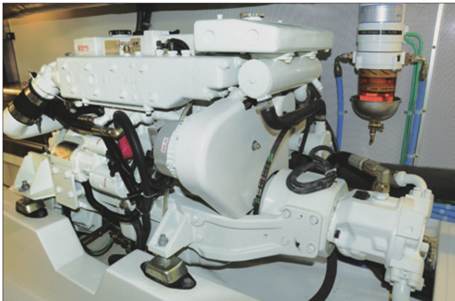
A tidy wing-engine installation like this one is a costly but effective get-home option. The relative accessibility of the secondary diesel power plant and its fuel supply system makes it more likely that the system will be well maintained, and in good working order if it is needed in an emergency.
