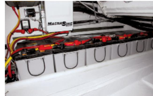
magnify the consequences, a battery adrift in an engine compartment, hydrogen gas accumulation within a battery box, or overheated and arcing connections are of great concern in any installation aboard any vessel, regardless of the bank's size.
