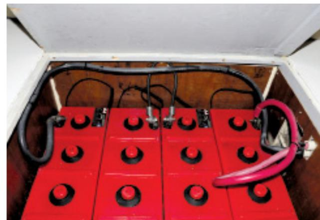
In order to allow hydrogen gas (which is lighter than air) to escape, ventilation ports must be located at the highest portion of the locker and/or box lid. This under-bunk installation fails to meet this requirement.
