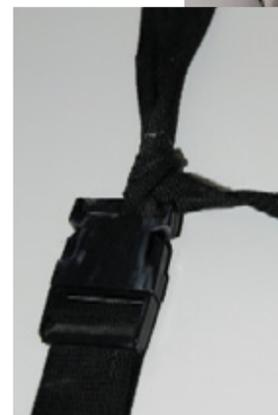
Top: The security of a battery installation is critically important for every vessel, however, the standard becomes more stringent where offshore passagemaking vessels are concerned. Left: Light-duty web straps have no place in battery security. This one, knotted to the buckle, is inadequate for even the smallest battery installation.
