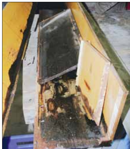
Wood battery boxes simply coated in resin cannot withstand exposure to acid. A coating applied without fabric reinforcement is too fragile for battery box construction.
