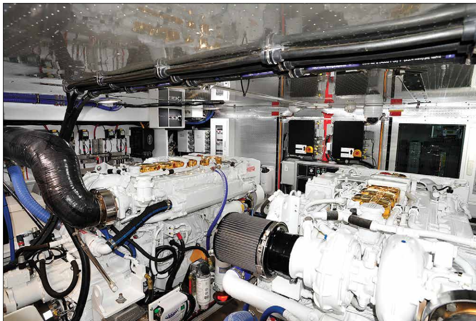
A pair of MAN R6 800-hp (600-kW) engines supplied by RDI and installed aboard a 58' (17.7m) semi-planing recreational cruising vessel. MAN builds marine engines for the commercial- and pleasure-boat markets. Since the recession, the former has become an increasingly important, and more reliable, sector for the manufacturer.
