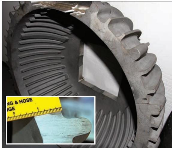
*Walls of the gyro's vacuum-chamber housing are reinforced cast aluminum, 1.25"-thick (32mm). The chamber allows the flywheel to spin freely, unimpeded by atmospheric resistance, and is strong enough to contain fragments of the flywheel should it disintegrate in motion.*
