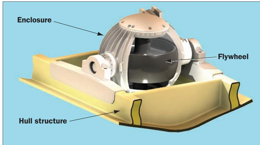
**Facing page**—Seakeeper's new gyroscopic stabilizer fits snugly under the cockpit sole of a Viking 43 (13m) sportfisherman. Vessel stability derives from a 400-lb (181-kg) flywheel spinning at 10,000 rpm inside a vacuum chamber. **Right**—Shepard McKenney, a principal investor in and developer of the Seakeeper gyro, discusses its technology in the company's research lab in Solomons, Maryland.
