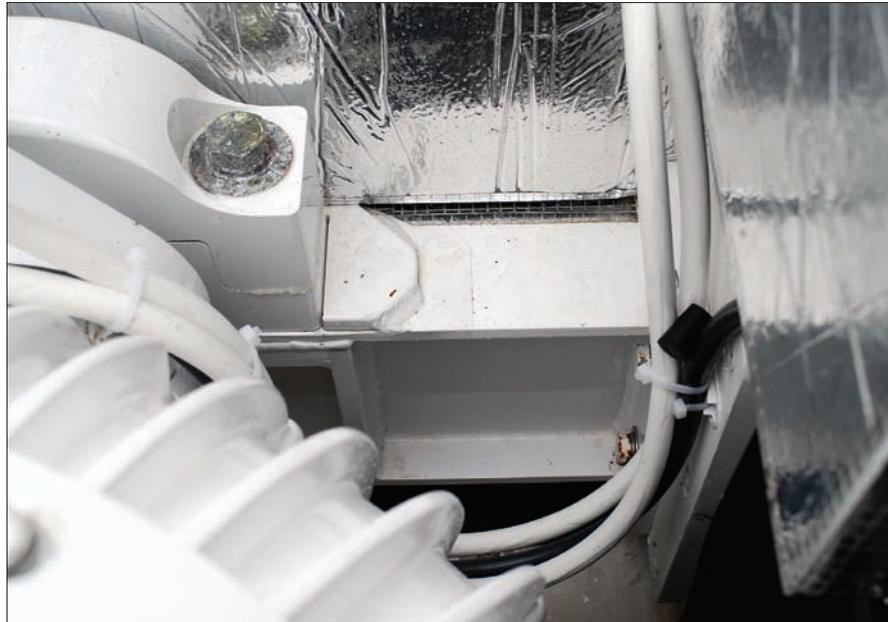
rounding structure to support the weight of the unit—just under 1,000 lbs (453.6 kg)—and the operating forces it exerts on a vessel. The vertical and horizontal torque applied to the hull can be roughly two tons in each direction. So, the gyro must be
