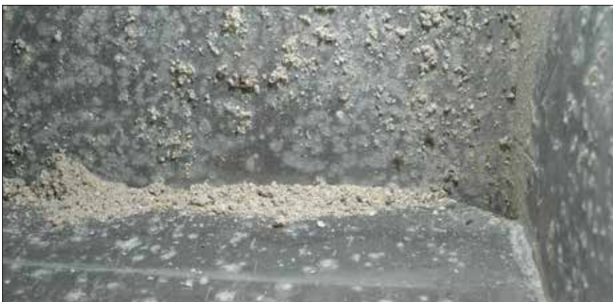
Aluminum's versatility doesn't extend to potable water applications, where the alloy is prone to corrosion, and often produces copious quantities of aluminum oxide—the white granular material shown here.
