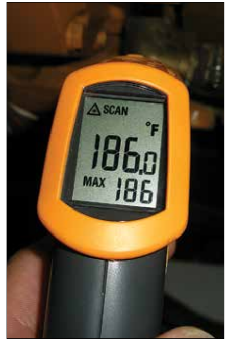
Above —Hot domestic water can cause serious burns, particularly if thermostats are set incorrectly, or if water is heated by engine coolant. In the latter case, mixing valves and anti-scald faucets can prevent dangerously hot water at the tap. Right —This infrared pyrometer is measuring the temperature of coolant as it enters a water heater.
