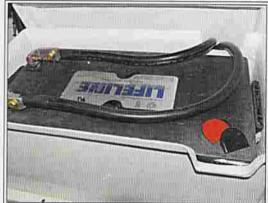
VRLA batteries lend themselves to less accessible installation options, and can even be installed lying on their sides (left). Dedicated VRLA/AGM start batteries (center) offer exceptionally high cold cranking amps (900 in this example) in relatively compact spaces. Even "sealed" AGM batteries (right) are capable of venting potentially explosive hydrogen, so their box lids must be equipped with vents at their apex.
