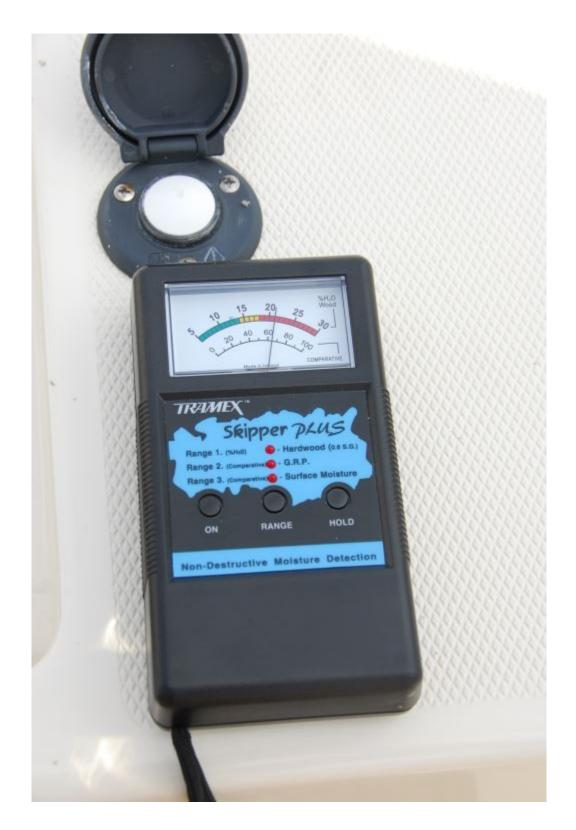
Cored composite construction is strong, light and stiff, it's been proven over many thousands of hulls. It is, however, susceptible to water entry at hull and deck penetrations, during or after the build. All penetrations on cored structures must be properly sealed in a process known as "close out". Sealant must *never* be relied upon to keep water out of core, and simply coating exposed core with resin is a
