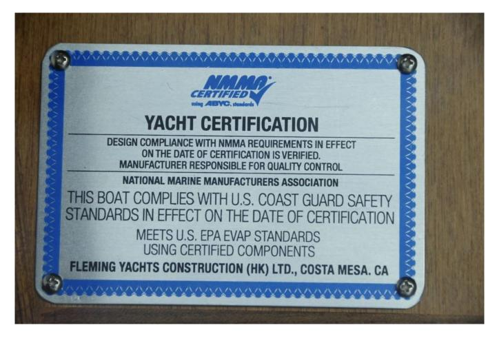
Vessels built to comply with third party standards can offer added value, reliability and safety. The standard or classification placard should be clearly visible.
