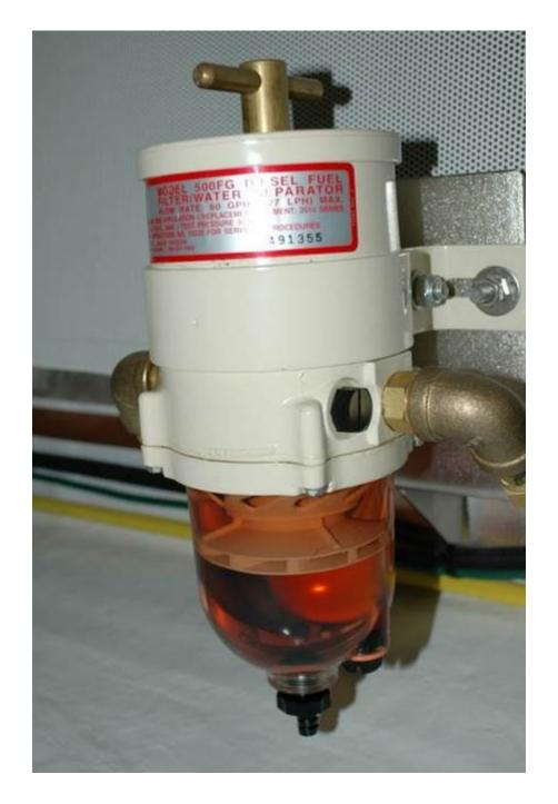
An FG series Racor turbine filter, installed aboard a new vessel. It *looks* good, so what's wrong with this set up? Plenty; FG series filters lack Underwriters Laboratories' (UL) approval for use in marine applications, which in turn means they do not comply with American Boat and Yacht Council (ABYC) standards for diesel fuel systems.
