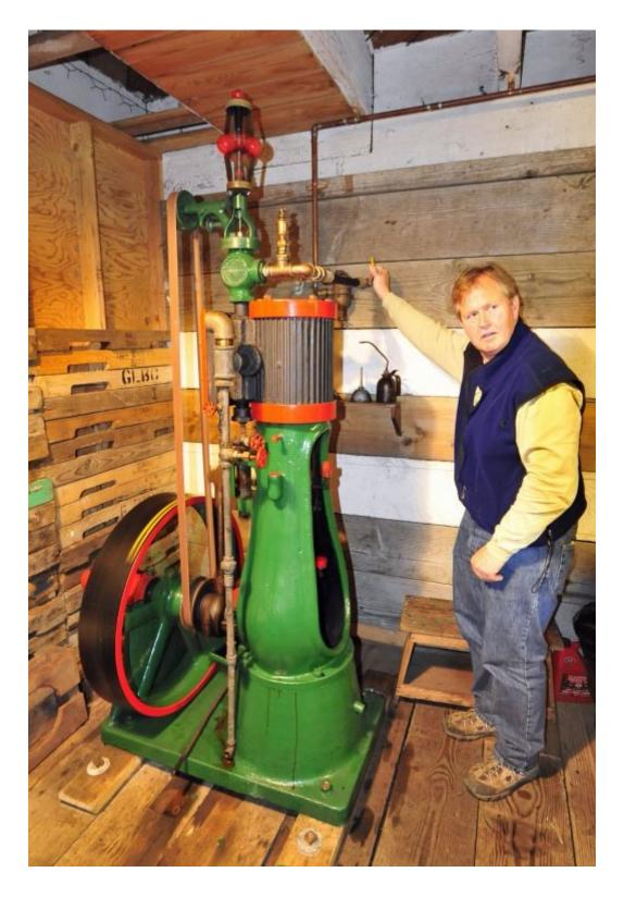
Alitak cannery manager Woody Knebel demonstrates his restored steam engine, which operates off the cannery's compressed air system.
