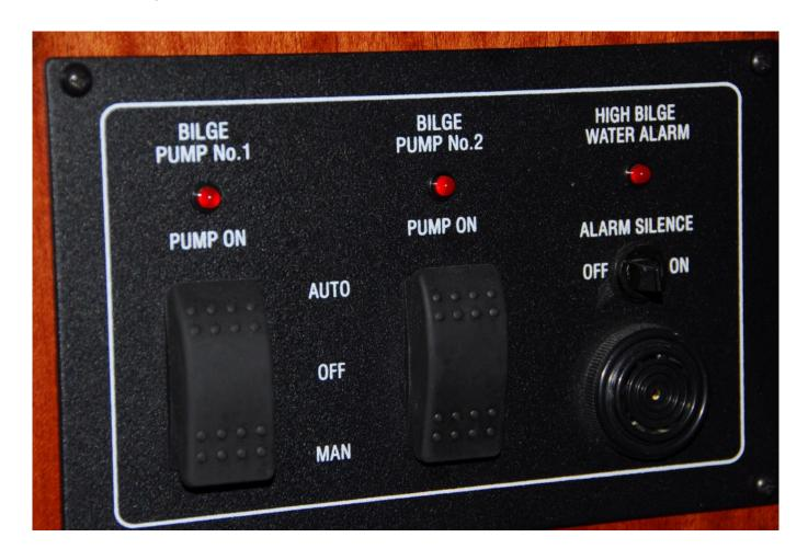
Paddle type switches are very easy to inadvertently turn off by accident, if you have this arrangement, they should be covered.
