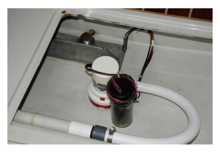
Bilge pump capacity and function should be tested often; this means actually adding water to the bilge, having it trigger both he high water alarm and pump switch, and allowing the pump to evacuate the water.
