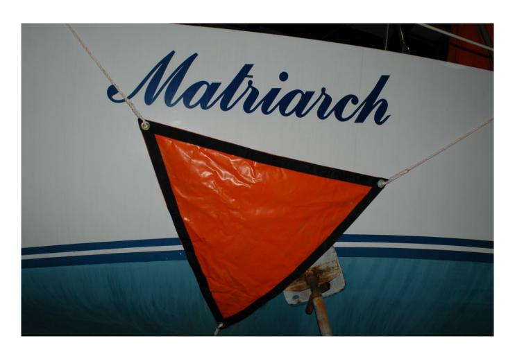
A fothering patch can be used to stem the flow of water, through hull damage from the outside. These can be challenging to use in anything other than calm conditions.
