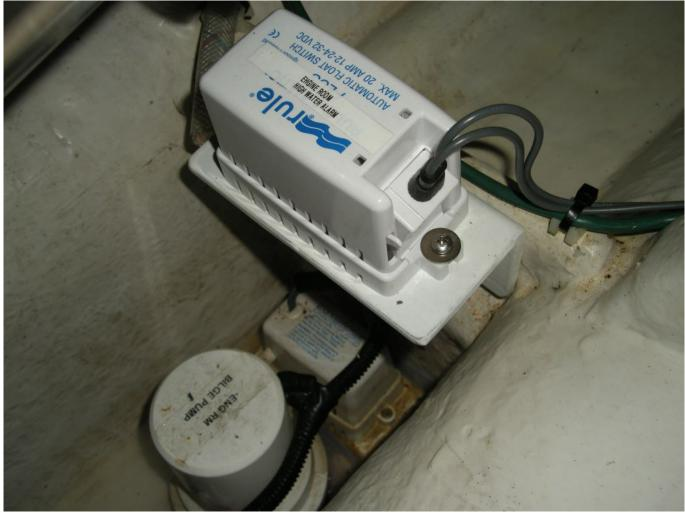
High water alarm floats should be placed to give the earliest possible indication of abnormal bilge water levels. Both of these are too high.
