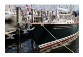
This cruiser has the right idea. With both a plow and a Bruce-style anchor (and a storm anchor in the lazarette), the boat is ready to take on most anchoring scenarios.
