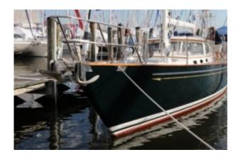
This cruiser has the right idea. With both a plow and a Bruce-style anchor (and a storm anchor in the lazarette), the boat is ready to take on most anchoring scenarios.
