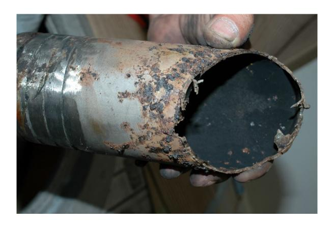
While exhaust risers and mixing nozzles are often made from 316L stainless steel, and more exotic alloys, failures are often a slow process, they begin with brown stains and weeping from welded joints. Failures can be a heartache, and expensive, however, rarely do they lead to uncontrolled flooding. Below the waterline components like exhaust outlets, and other submerged fittings and plumbing, are on the other hand, an entirely different matter. A failure here nearly always results in flooding.
