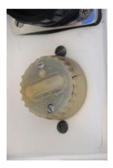
These fuse holders were common on some makes of boats, but they don't meet ABYC standards for over current protection of the incoming AC wiring because if the fuse were to blow, it wouldn't trip both the hot and neutral lines simultaneously.
