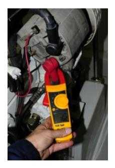
This multimeter is indicating that the alternator is producing
