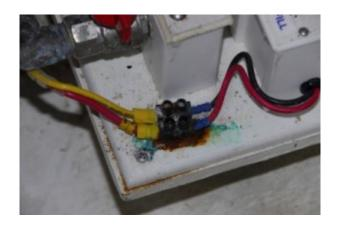
Water dripping on an electrical connection can cause corrosion which can lead to a high resisitance, high heat problem, but not necessarily a dead short. Any junction as poor as this should be replaced immediately.
