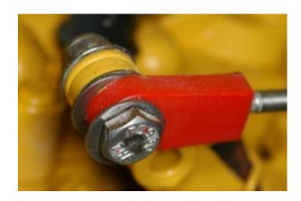
Failing to use the right, manufacturer-specified parts for the job is a frequent oversight attention to detail faux pas. Here, a common nut and bolt, rather than the purpose made pivot pin, has been used to secure a throttle cable to an injection pump aboard this new boat.
