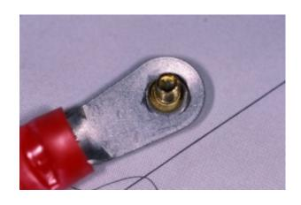
Electrical systems frequently fall prey to poor attention to detail. In order to convey current with minimal resistance, holes in ring terminals, and the fasteners that secure them, must be the same size.
