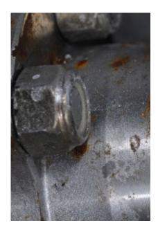
The fasteners that secure this propeller shaft coupling to the transmission have loosened, because they are uniformly too short to engage the nuts' nylon locking ring inserts.
