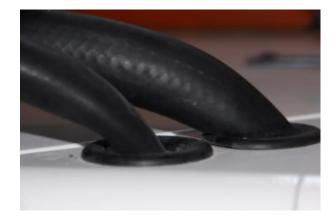
This newly installed generator overheated shortly after it was first started. The cause; hose with insufficient wall stiffness that collapsed when passed through the sound enclosure.
