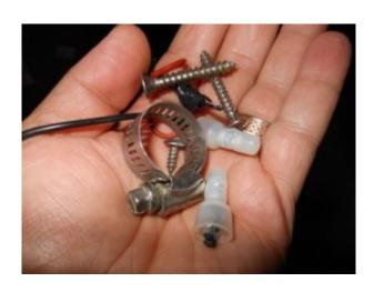
On its own, bilge debris may be dismissed as an annoyance or simply sloppy. Yet, it may have serious consequences if, for instance, it's drawn into and clogs a bilge pump.
