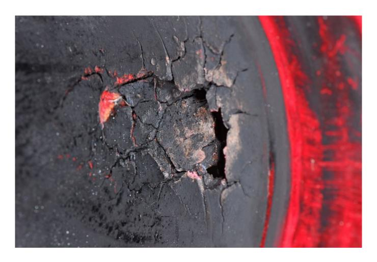
Wet exhausts require a continuous flow of cooling water. If it's lost, even for a few seconds, the exhaust system hose, plastic and fiberglass components will quickly overheat; in a worst case scenario it could catch fire.
