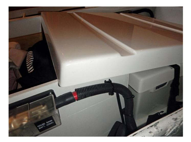
This nicely-made fiberglass battery box has one fatal flaw; the lid forms an envelope in which hydrogen gas can become trapped. A few small holes in the top will easily remedy this problem.
