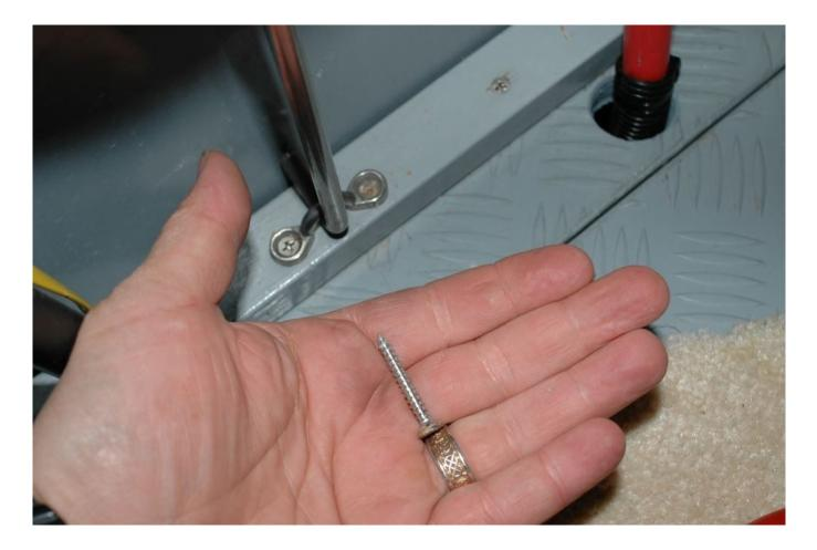
Battery support hardware should be retained with through bolts. If tapping screws must be used they should be the largest/longest that will be accommodated by the hardware and substrate.
