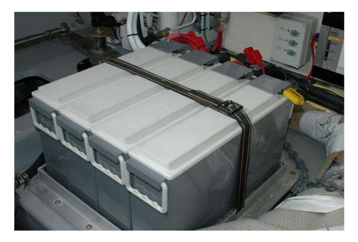
Batteries that fit tightly within a box, or strapped together side by side, are a double-edged sword, they may not move as much, however, ventilation between batteries is compromised.
