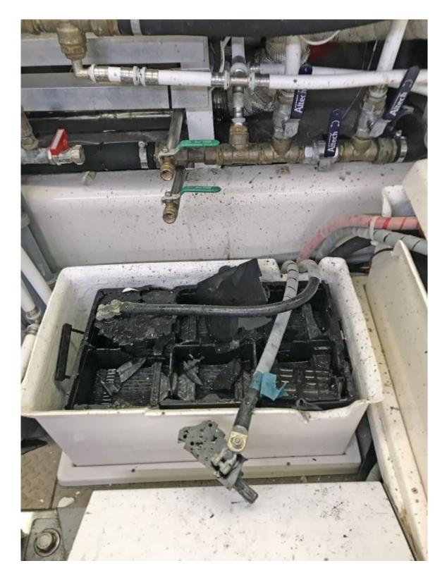
Flooded batteries do occasionally explode, like the one shown here. For that reason, full enclosure within a box does make good sense.
