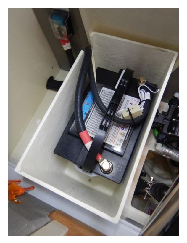
This battery box is too large for the battery (or the battery is too small for the box). Shims are needed to prevent it
