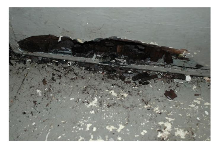
Raw or painted timber is unsuitable for battery box material, it is quickly destroyed by leaking electrolyte.
