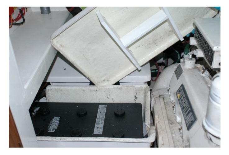
This battery box is secured with heavy duty straps, and shims have been attached to the inside of the lid to retain the battery.
