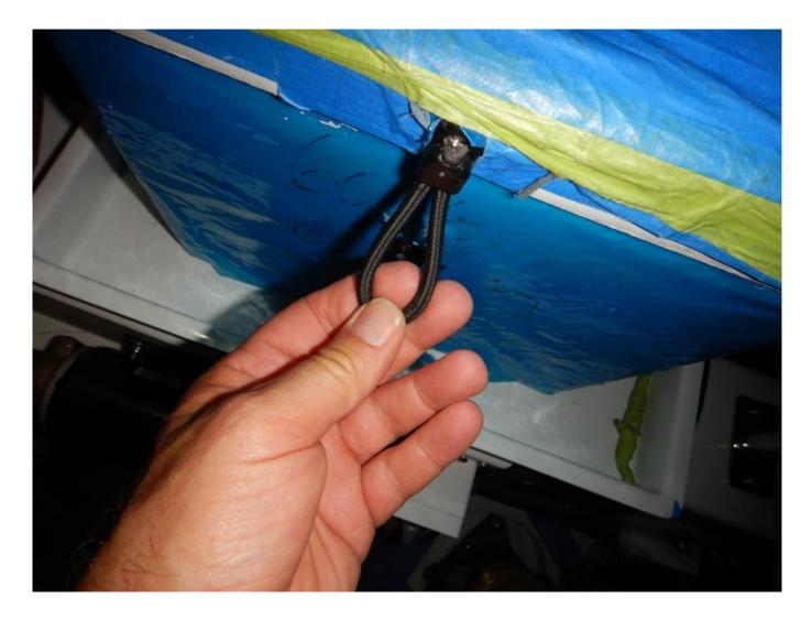
The elastic straps that hold this battery box's lid in place, and which are expected to keep the battery secure and stable within the box, are simply inadequate for the task.
