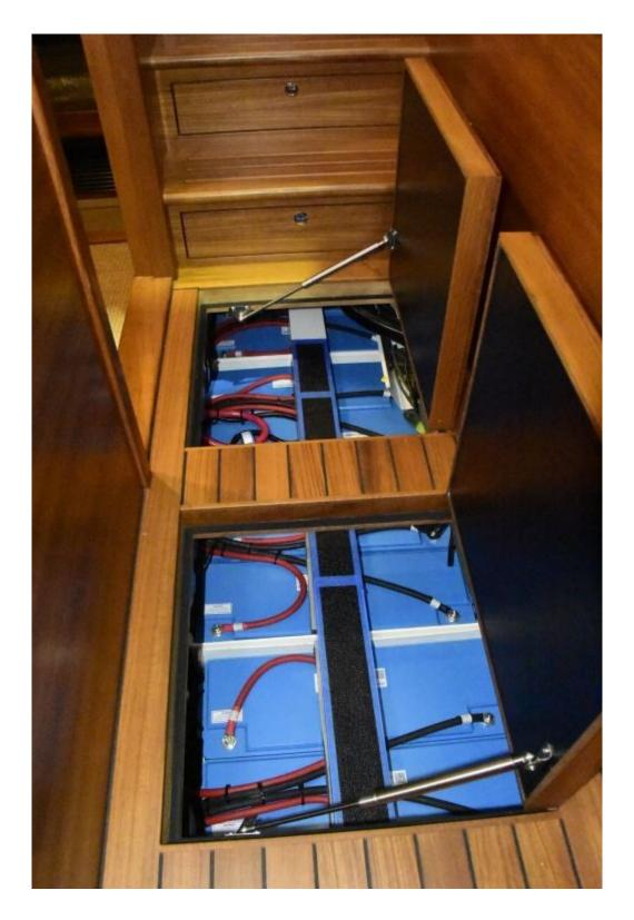
This Lithium Ion battery bank is retained by a single clamptype strong back. The positive terminals should be insulated.
