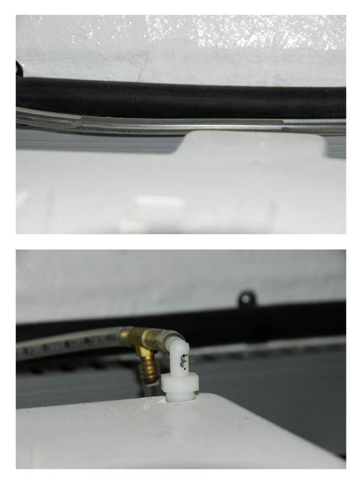
This battery box has been equipped with a remote ventilation
