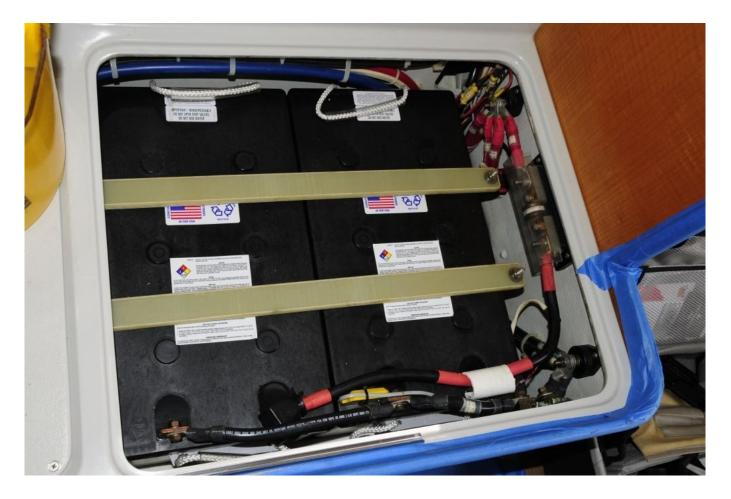
A textbook battery installation, these batteries are securely clamped in place and will resist even the most violent sea
