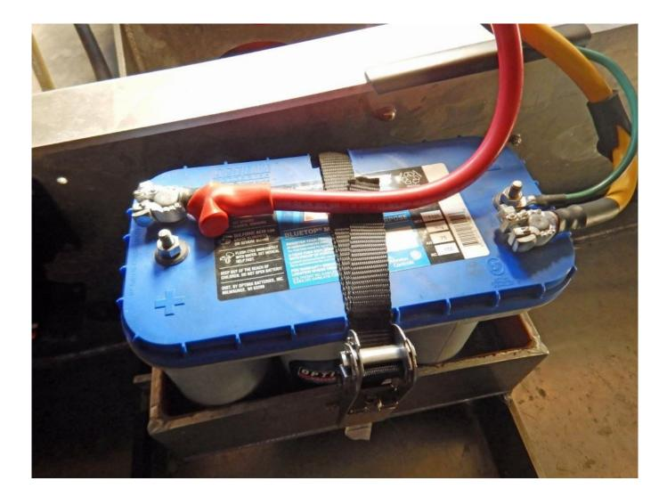
Heavy duty ratcheting straps, with stainless buckles, can be used very effectively for battery hold-downs (the positive terminal on this battery should be insulated).
