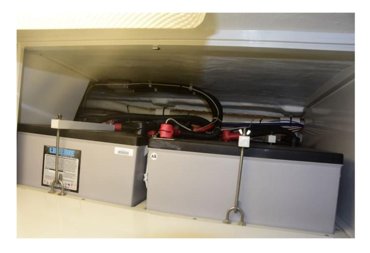
Clamp arrangements prevent all battery movement, and are therefore ideal; note the heavy through-bolted eye bolts.
