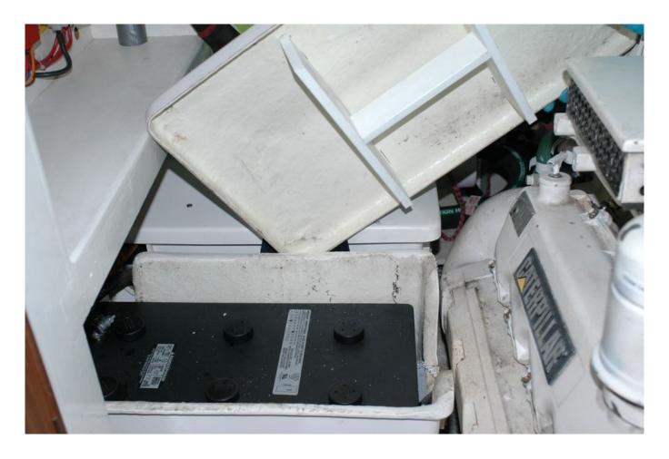
This battery box is secured with heavy duty straps, and shims have been attached to the inside of the lid to retain the battery.
