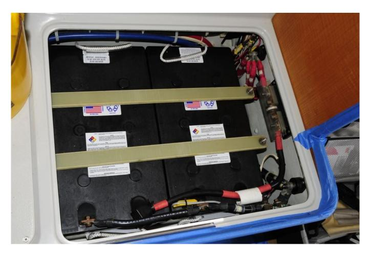
A textbook battery installation, these batteries are securely clamped in place and will resist even the most violent sea
