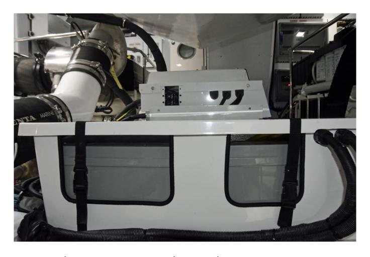
A box with large holes cut in the side somewhat defeats the purpose of containment. For flooded batteries boxes can make sense, otherwise their benefit is questionable.
