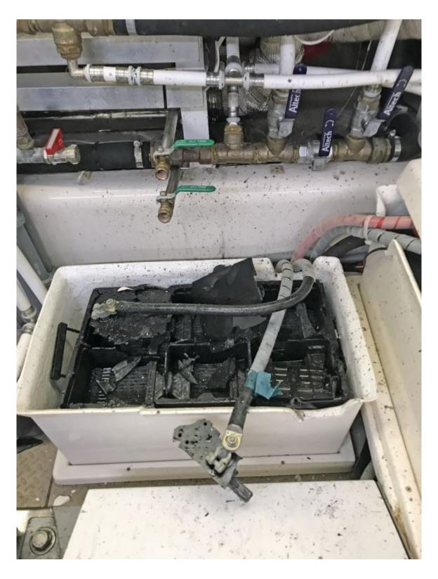
Flooded batteries do occasionally explode, like the one shown here. For that reason, full enclosure within a box does make good sense.
