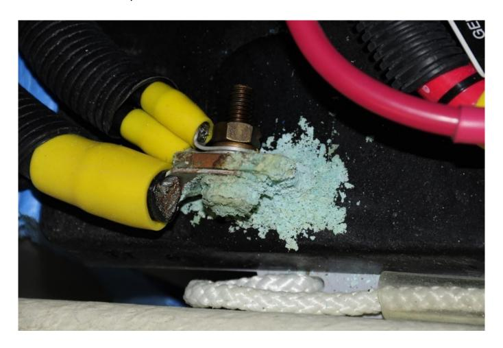
Installing batteries in boxes makes casual inspection impossible. As a result, problems like this corroded post are likely to linger until a failure occurs.
