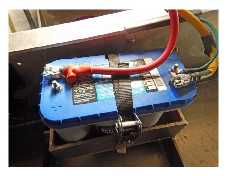
Heavy duty ratcheting straps, with stainless buckles, can be used very effectively for battery hold-downs (the positive terminal on this battery should be insulated).
