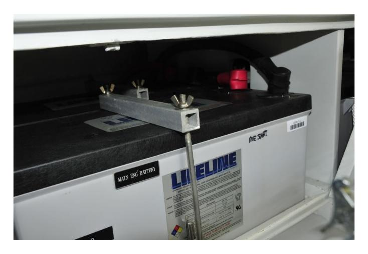
To prevent the possibility of short circuits, the material used for the clamp strong back should be non-metallic; the one shown here is extruded fiberglass.
