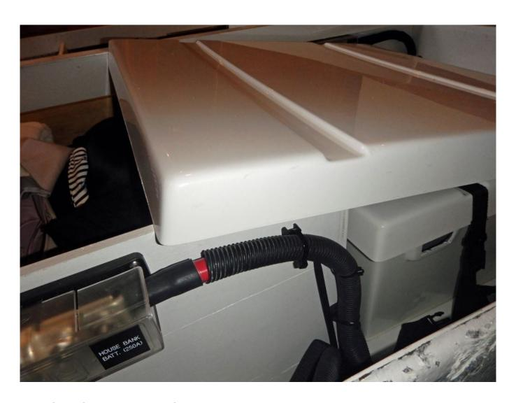
This nicely-made fiberglass battery box has one fatal flaw; the lid forms an envelope in which hydrogen gas can become trapped. A few small holes in the top will easily remedy this problem.
