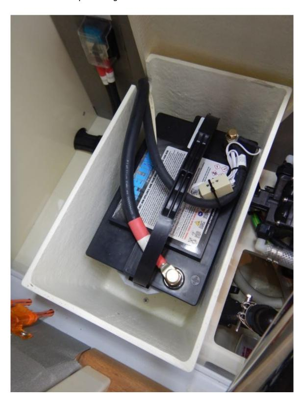
This battery box is too large for the battery (or the battery is too small for the box). Shims are needed to prevent it
