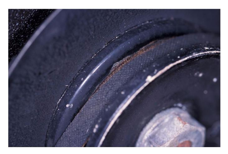
This belt is far too narrow for its pulley, it's riding in the bottom of the groove, where contact is limited.
