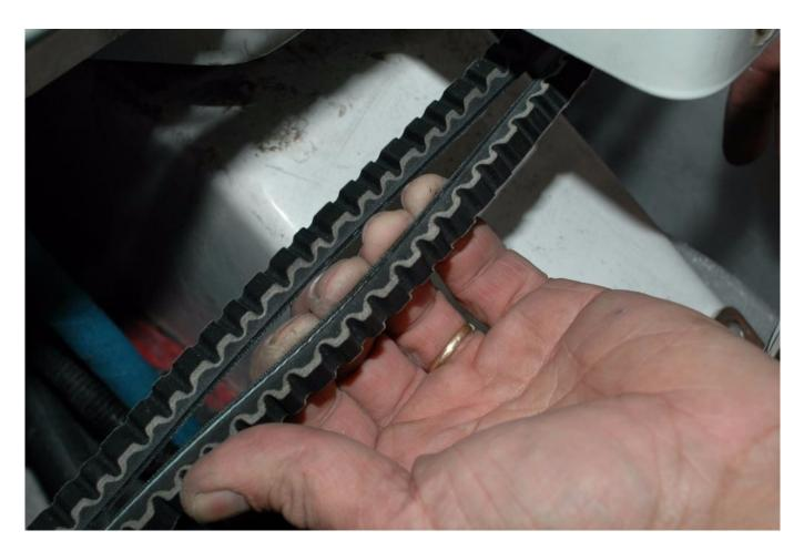
Notched belts are well suited to small diameter pulleys. Using them reduces the likelihood of belt overheating, which is caused by rapid flexing of conventional belts.
