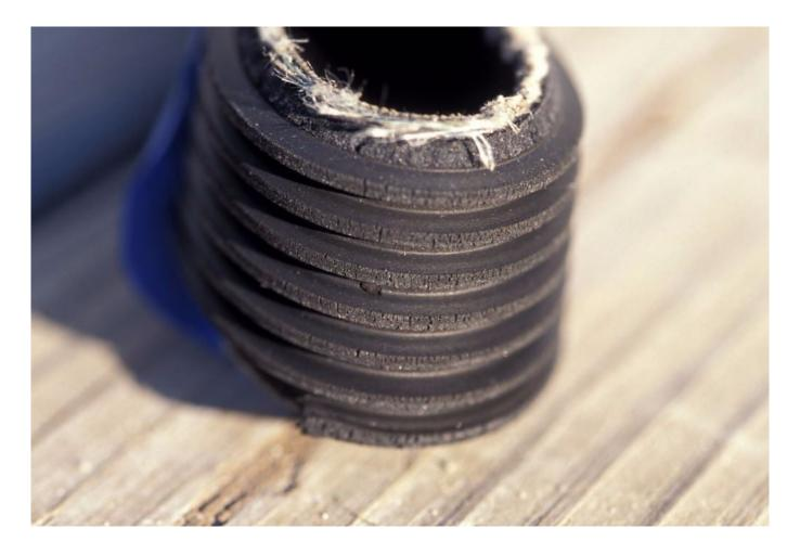
This serpentine belt is suffering from both wear and tear, as well as a worn tensioning pulley. The latter is evidenced by the white filament visible on this belt, the result of misalignment induced by the worn tensioner.
