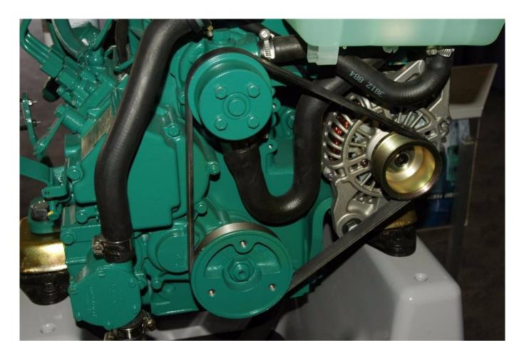
While most serpentine belt-equipped engines rely on an automatic tensioning device, some smaller models continue to utilize the alternator's adjustment for tensioning purposes.
