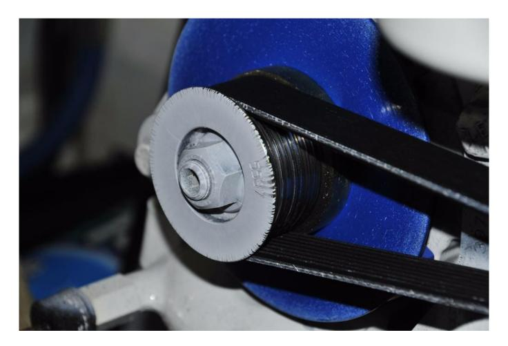
Belt engagement is critical, particularly on highly loaded components such as high output alternators. The rule of thumb for these is no less than 120°. Shedding of belt chips, or chunks can be a sign of a heavily loaded belt that lacks sufficient pulley engagement or tension, which can cause the belt to skip; this is also especially common on high output alternator installations, where belts should engage pulleys for a minimum of 120°.
