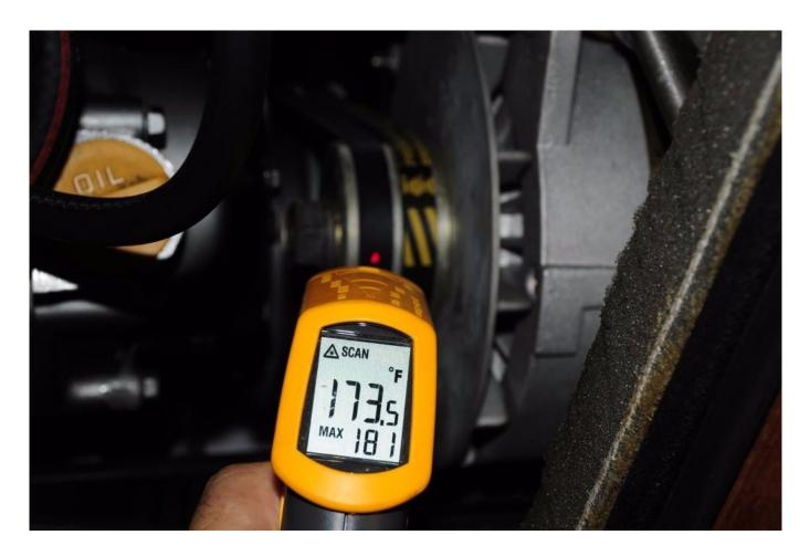
A properly selected and tensioned belt typically runs at roughly the same temperature as the engine's coolant, between 175°F and 200°F.
