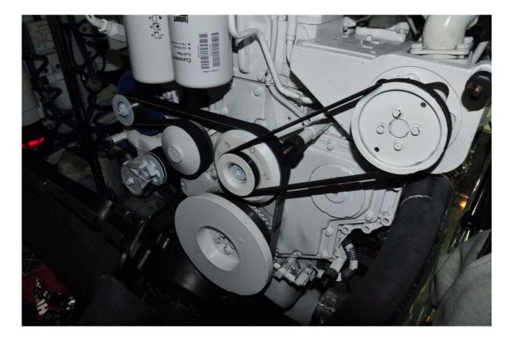
While nearly all belts are installed either by adjusting a driven pulley's position, an alternator or pump for instance, or by compressing a self-tensioning device, some like the one shown here (upper right) rely on "rolling", where the belt is simply stretched over a pulley by rotating the latter.
