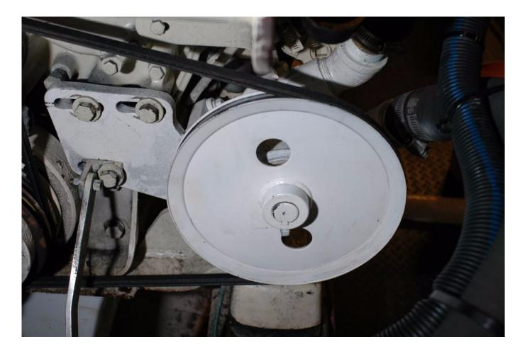
Large diameter pulleys engage the belt over considerable surface area, making slippage unlikely even when belts are under tensioned.
