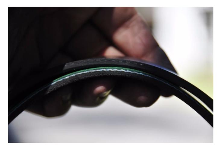
Demanding applications require heavy duty belts. The Gates FleetRunner series, available in both V and serpentine style, used on ambulances, emergency and military vehicles, is well suited to marine high output alternator applications. Compared to conventional belts, they are thicker and include additional reinforcement.
