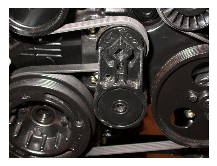
Many serpentine belt systems rely on an automatic or selftensioning pulley. Most utilize a square recess, one can be seen here in the center of this image, into which a socket drive or breaker bar is inserted, which in turn is used to compress the spring for belt replacement.
