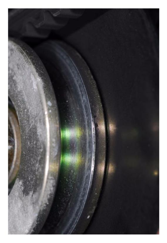
This belt is too wide for the pulley its driving, the belt stands substantially proud of the pulley, and it fails to make contact with most of the pulley wall, which can be seen by the wear pattern that is too high up the grove wall. Ideally, the wear pattern should be centered on the pulley wall.
