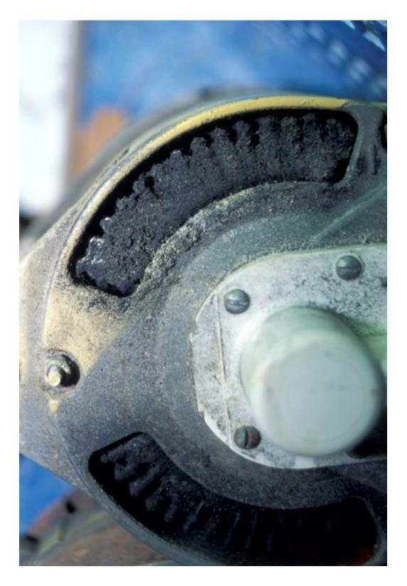
Belt dust, which is frequently generated by misaligned belts, is extremely fine. In addition to distributing itself over the front of the engine, it's also drawn into the alternator, where it is deposited, and interferes with heat dissipation, as well as the engine's air intake.
