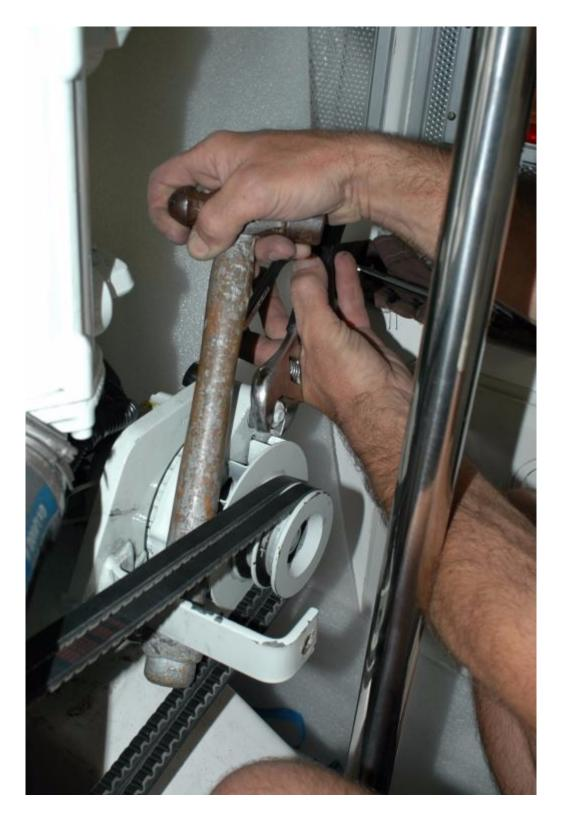
The handle of a hammer can be used to push an alternator or pump away from the crankshaft pulley, thereby tensioning the belt for adjustment.
