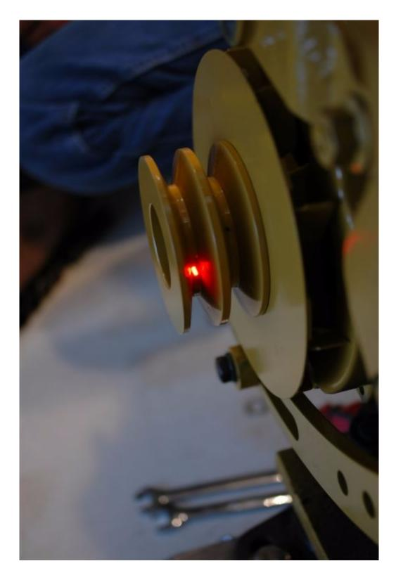
A laser is being used here to confirm proper belt alignment for this alternator, one of three on this engine.
