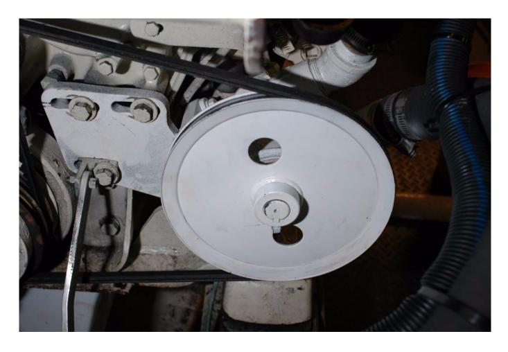
Large diameter pulleys engage the belt over considerable surface area, making slippage unlikely even when belts are under tensioned.
