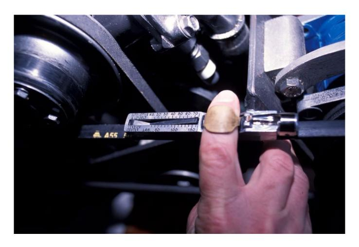
A Gates "Krikit" belt tension gauge, which enables users to apply proper tension to V belts.
