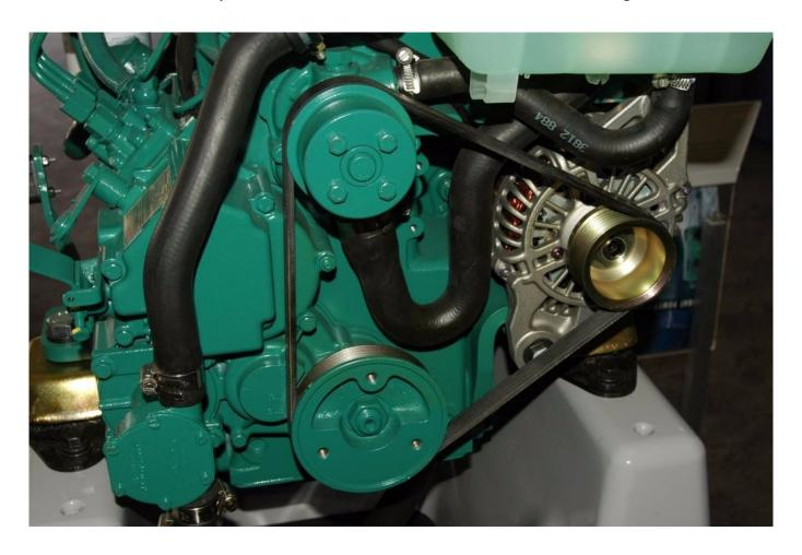
While most serpentine belt-equipped engines rely on an automatic tensioning device, some smaller models continue to utilize the alternator's adjustment for tensioning purposes.
