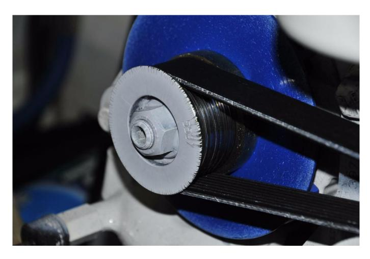
Belt engagement is critical, particularly on highly loaded components such as high output alternators. The rule of thumb for these is no less than 120°.
