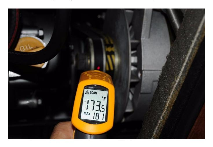
A properly selected and tensioned belt typically runs at roughly the same temperature as the engine's coolant, between 175°F and 200°F.
