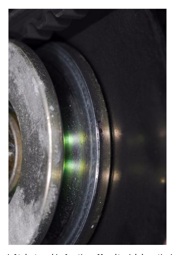
This belt is too wide for the pulley its driving, the belt stands substantially proud of the pulley, and it fails to make contact with most of the pulley wall, which can be seen by the wear pattern that is too high up the grove wall. Ideally, the wear pattern should be centered on the pulley wall.
