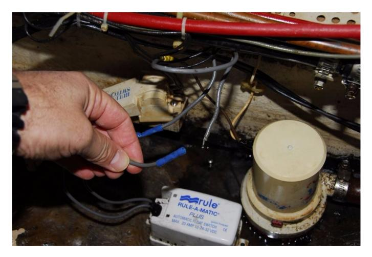
Bilge pump wiring and terminations must be rugged and robust. If connections can't be made at least 18 inches above the base of the pump, they should be water-proof. If they can be easily pulled apart, like the one shown here, there's a good chance the installer lacked the necessary skills to properly use a crimping tool. Without a doubt, connections this close to bilge water must be waterproof.
