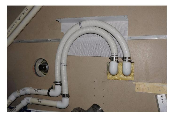
These installations carry with them a series of insidious and serious faults, including and especially risers without antisiphon valves (above and top), and paralleled pump discharges (top). While risers effectively prevent down flooding, they do nothing to mitigate siphoning.
