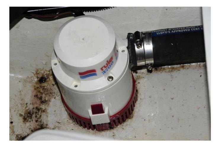
For high capacity in a small package, submersible pumps are the obvious choice.
