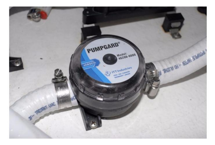
For bilge drying, a self-priming diaphragm type pump (top and middle) is often the best choice. Located well above bilge water, its pick up hose can remove water to a lower level than a submersible pump. Such pumps are sensitive to debris ingestion, and as such they must be equipped with in-line strainers (above).
