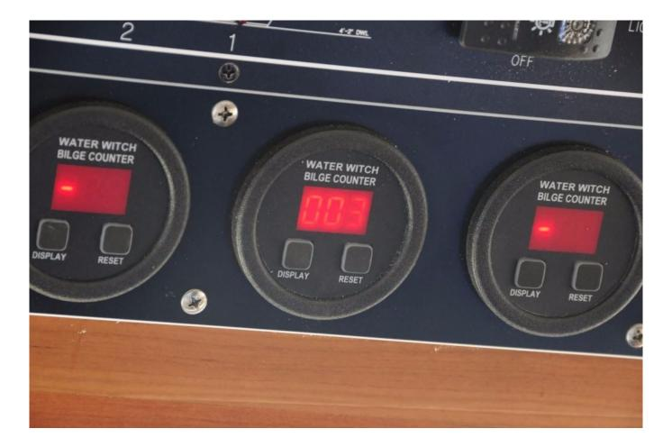
In addition to a 'pump on' indicator light, bilge counters can be an invaluable addition to any bilge pump installation.
