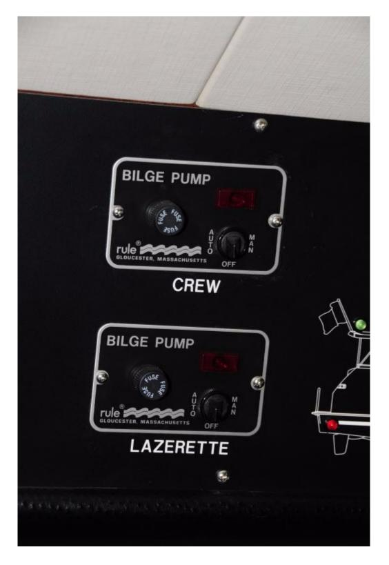
While familiar and functional, the 'momentary on' switch panel with fuse is less than ideal. Circuit breakers are preferred, as are continuous on switches.
