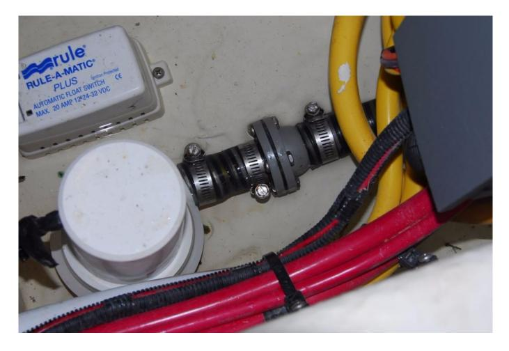
Check valves are commonly found on bilge pump installations. They are a tempting remedy for preventing water contained in a long hose run from sluicing back into the bilge, however, they are not without their liabilities.
