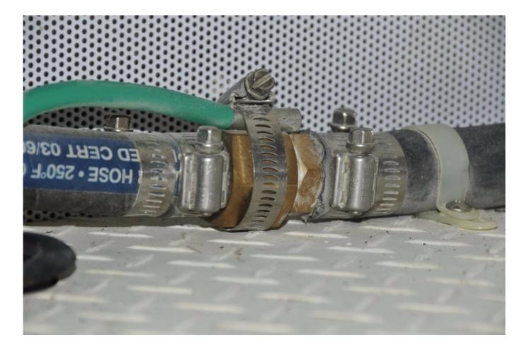
Bonding otherwise isolated metal plumbing components that carry seawater is of limited value. However, there's no harm in doing so in spite of the fact that they are too far away from any anode to derive protection. In rare instances such bonding may be prevent stray current corrosion. Note the approved method used to make the connection, a barrel terminal
