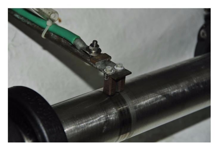
Bonding wires should be attached directly to shaft brushes, this wand style is correctly wired, rather than to the fasteners that support the wand to which they are mounted.
