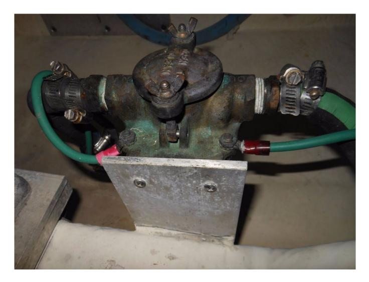
Connecting bonded items in series, also known as "daisy chaining", should be avoided as it adds unnecessary resistance to the circuit. Ideally, each bonded item should be connected directly to a bonding bus bar.
