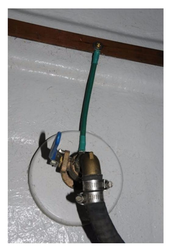
The "drop" or "home run" method of bonding connection, wherein each bonded object is connected directly to a copper bus bar,
