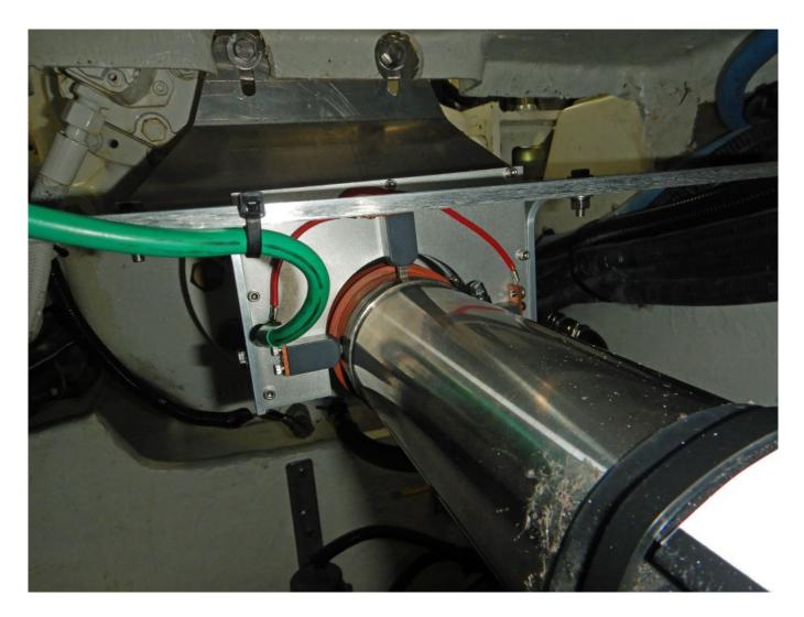
A high quality, and very effective, multi-brush, silver slip ring shaft brush assembly. If the shaft must be bonded, it must be with a very low resistance connection; this is the most reliable means of achieving that end.
