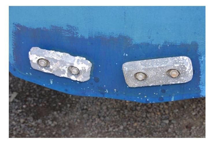
Uneven consumption of anodes is often a clear indication of a compromised bonding system.
