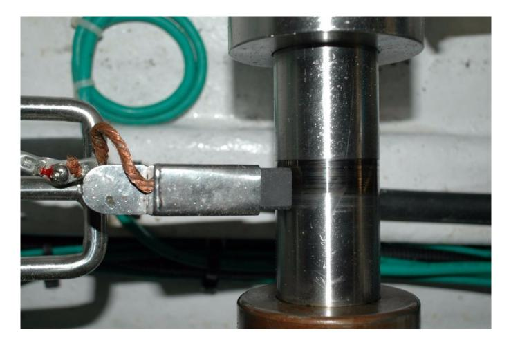
There are shaft brushes and there are shaft brushes, the one shown here relies on a spring-loaded carbon electric motor commutator brush, which is preferred. However, it still has
