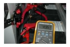
Although it will not test a battery's ability to deliver amperes, a high quality multimeter, such as the one shown here, will enable you to determine a battery's state of charge provided it's been, "rested". Based onthe voltage of 12.35, this AGM battery is more than 50% depleted.
