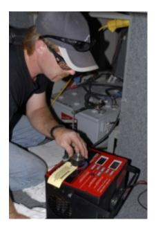
Carbon pile load testers, like the one shown here, place a heavy load on the battery in order to simulate high ampere consumer scenarios such as starting or inverter use. Safety goggles should be worn when ever working with batteries, regardless of whether they are flooded, AGM or gel.
