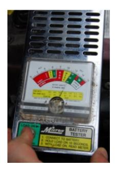
A resistive load tester such as the one shown here, sometimes referred to as a, "toaster" can be effectively used to determine the condition of many smaller starting batteries, however, its accuracy for large, deep cycle batteries is less certain. At left is the battery's voltage without a load present, while on the right the load has been applied and the battery is carrying it without difficulty.
