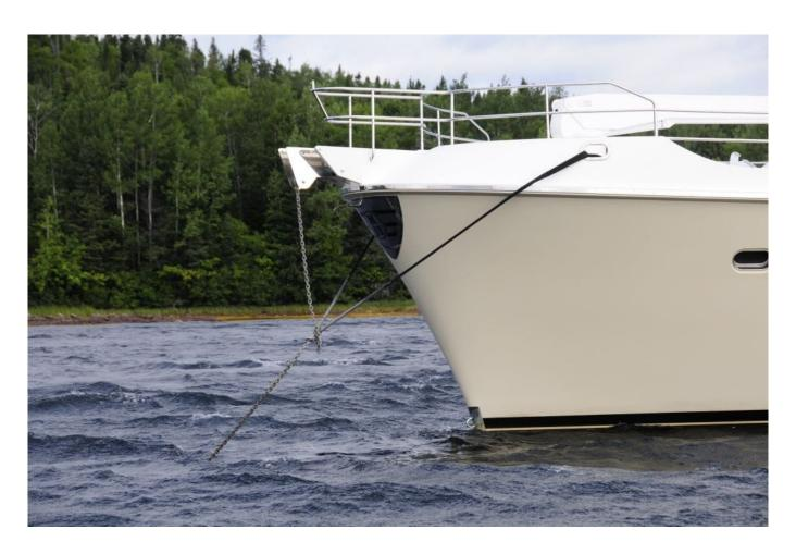
It doesn't take much wind to pull this expedition trawler's chain bar tight, even in a protected anchorage. It is here that a properly designed and deployed snubber system demonstrates its value.
