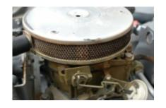
Gasoline engines produce CO. The less efficiently they are operating, the more CO they produce. Therefore, engines in poor tune or those that are inefficiently loaded produce more CO. Engines equipped with carburetors, like those shown above, as opposed to fuel injection, are more likely to be out of tune or have poor mixture and thus they are more likely to produce excess CO. However, all internal combustion engines produce CO and therefore should be considered sources of this
