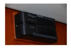
CO detectors are available in a variety of shapes, sizes and colors. The most desirable feature is their cost, they are inexpensive and thus there's no reason for not having one or more aboard. Most importantly, they must be replaced in accordance with the manufacturer's quidelines.
