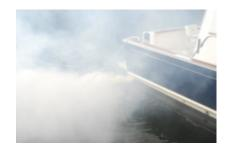
The presence of smoke, or lack thereof, is not a determining factor for the presence of CO. Engine's whose exhaust is invisible to the naked eye can and often do produce lethal concentrations of CO.
