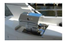
Don't rule out the gas grill as a CO source, particularly if used in a curtained or enclosed bridge area. Ensure sufficient ventilation, particularly if a bow-on wind is creating a station wagon effect, which often occurs for vessels at anchor.
