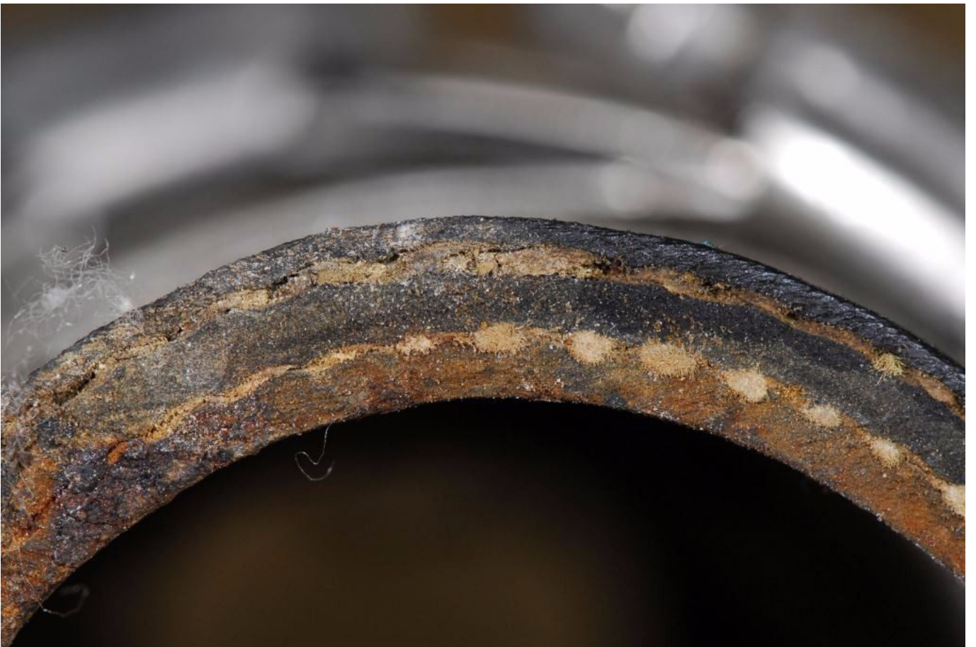
The five plies of a stuffing box hose (top) are clear to see,
