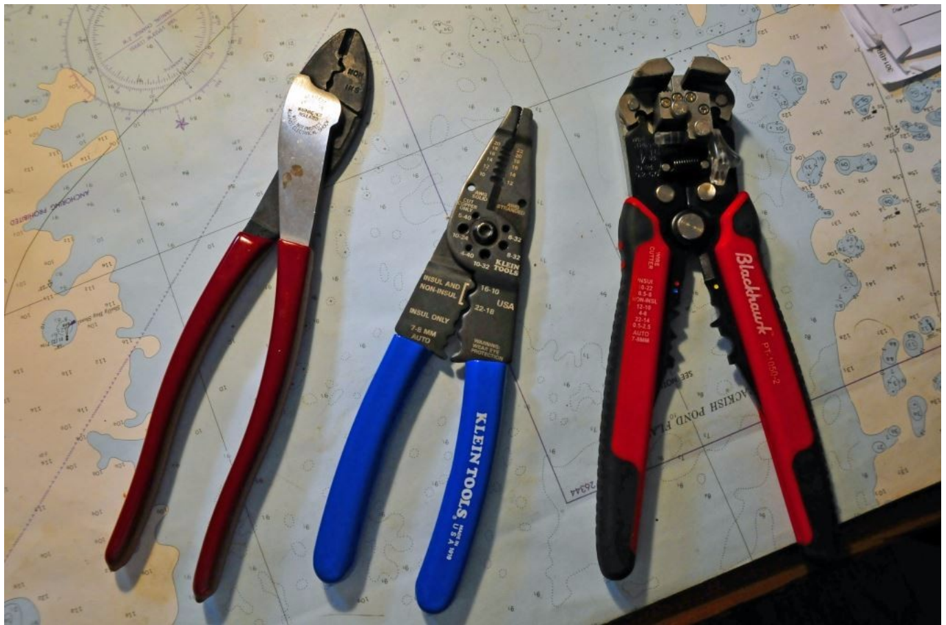
Preferred hand tools L to R, conventional crimpers, manual strippers (which also crimp inboard of the pivot), and automatic strippers.
