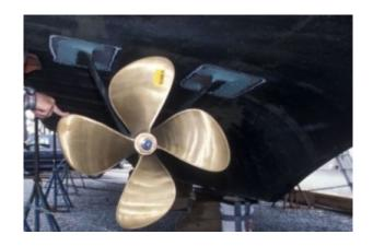
While not necessarily definitive, the ease with which a propeller can be turned while a vessel is hauled can be an indicator of shaft to bearing fit and alignment.
