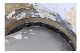
This bearing has swollen, there is no gap between it and the shaft, making the shaft both difficult to turn and prone to accelerated wear.
