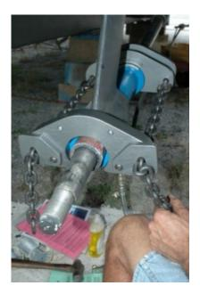
There are several ways to remove shaft bearings. Here, a hydraulic split drift removal tool is being used. While costly, on the order of \$2500 at the time this was written, they make bearing removal easier in that the shaft does not require removal.
