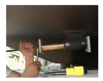
A mechanical bearing installation tool made using a length of threaded rod and two sections of aluminum plate. This technique is easy on the strut and often works well. The alternative, and one that is frowned upon, involves using a mallet to drive the bearing into the strut.
