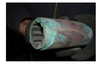
The metallic shell used for shaft bearings is often made of a brass alloy. Becuase brass alloys contain zinc they are prone to galvanic corrosion. This can be prevented with proper anodic protection, i.e. use of zinc or aluminum anodes. However, it's important to keep in mind that the shell is somewhat sacrificial, it's designed to corrode before the more valuable strut, and is more easily replaced.
