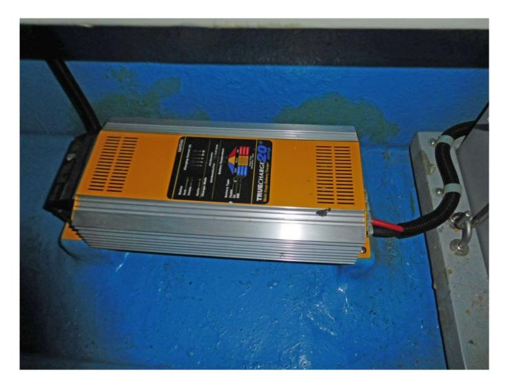
Battery chargers and similar electrical equipment should be mounted well above bilge water. While this unit rests on pedestals, they lack adequate height above the potential accumulation of bilge water; in this case another location should eb chosen.
