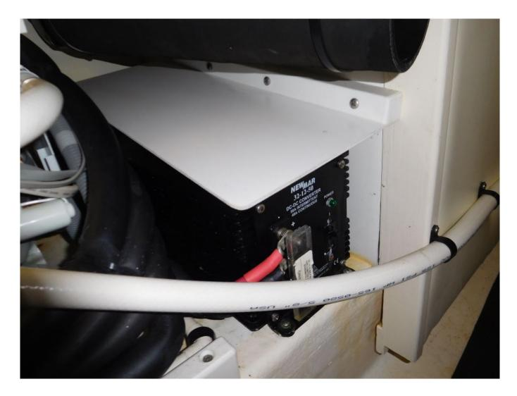
This DC to DC converter could be considered a battery charger of sorts; it is equipped with a drip shield.
