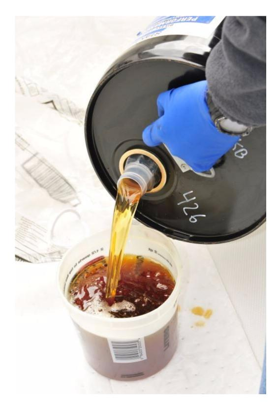
A lubricity and cetane enhancer being measured aboard a cruising vessel taking on fuel in Greenland. Because the quality of fuel both at home and abroad is never certain, using a lubricity additive is reasonable and represents a belt and suspenders approach.
