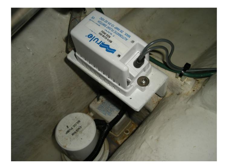
High water alarm switches must be located so that they provide the earliest possible indication of flooding; that usually means no more than just a couple of inches above the primary pump's switch. The one shown here is, once again, too high.
