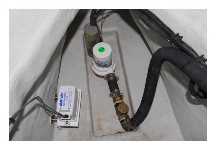
Located only slightly above the switch for the pump, this high water alarm float switch is properly located.
