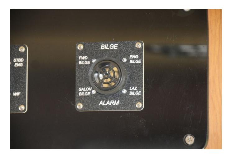
This high water alarm annunciator is well-designed, it includes a single audible horn, and indicator lights to show which compartment is flooding.
