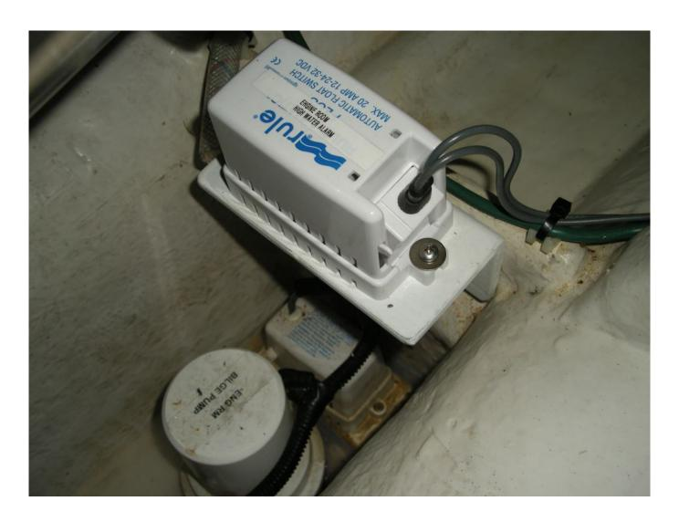
High water alarm switches must be located so that they provide the earliest possible indication of flooding; that usually means no more than just a couple of inches above the primary pump's switch. The one shown here is, once again, too high.
