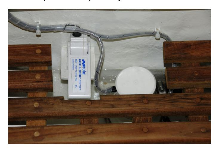
This high water alarm switch is located above the bilge pump, it's too high and in this case vulnerable to being stepped on.
