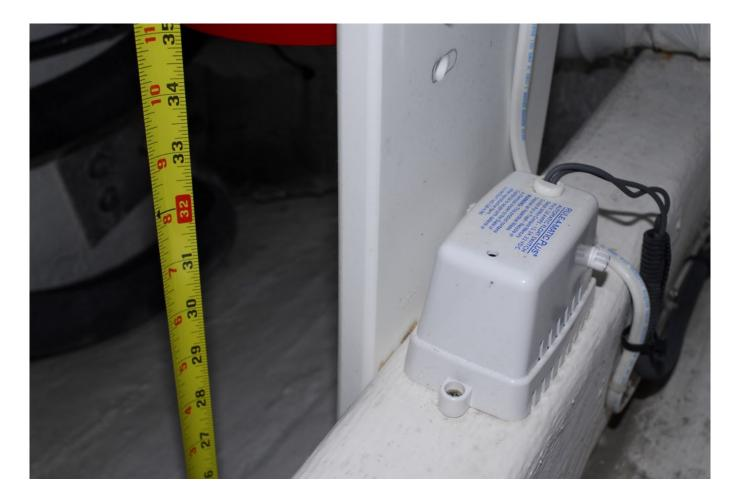
This high water alarm, located on an engine bed stringer, is over 30-inches above the bilge pump, and above the bottom of the engine.
