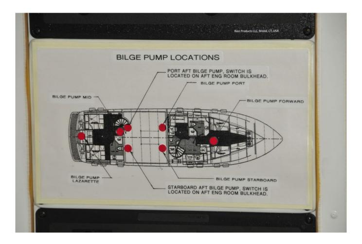
A chart showing seacock and bilge pump locations makes good sense, make certain the font can be easily read in a low-light, emergency scenario.
