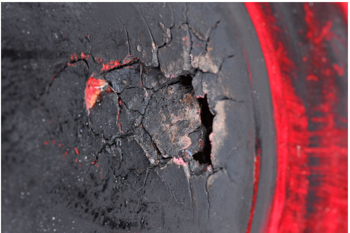
This wet exhaust hose was burned, and ultimately pierced, when
