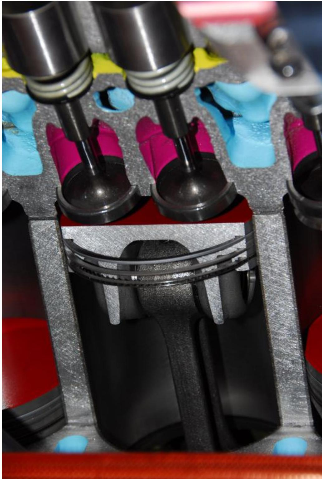
**Without properly functioning piston rings, it would be impossible to generate sufficient compression to support diesel combustion. When rings leak or otherwise fail, the results can be hard starting, smoking, poor fuel economy and reduced power.**
