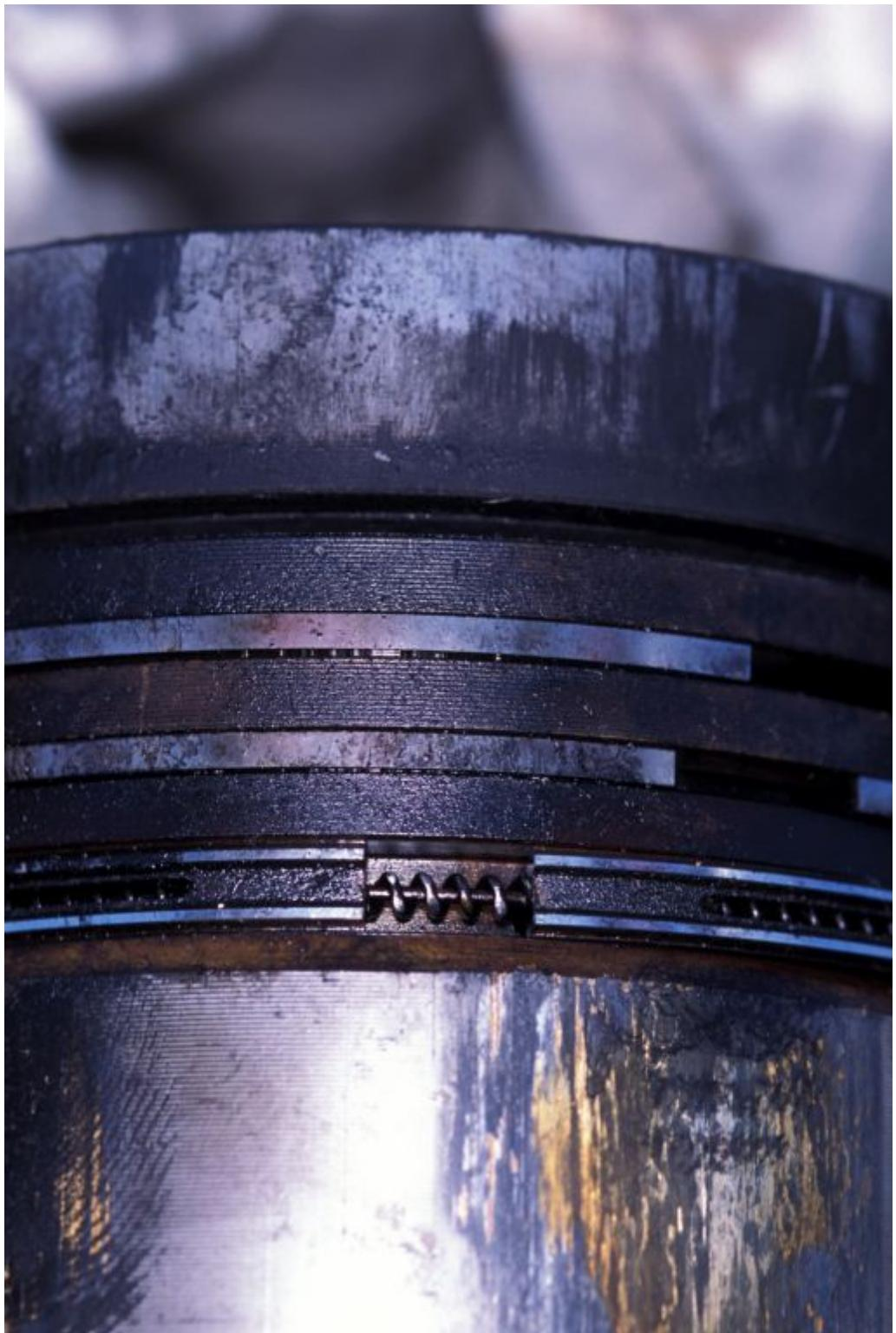
Piston rings typically include a set of two compression rings, top in this image, and an oil control ring, which in this case is a single, one-piece ring, which is installed over an expansion spring. The latter ensures the ring maintains even pressure on the cylinder wall for the most effective oil scraping. In this case, this image represents a very worn set of rings that appears quite wet with diesel fuel or oil. High
