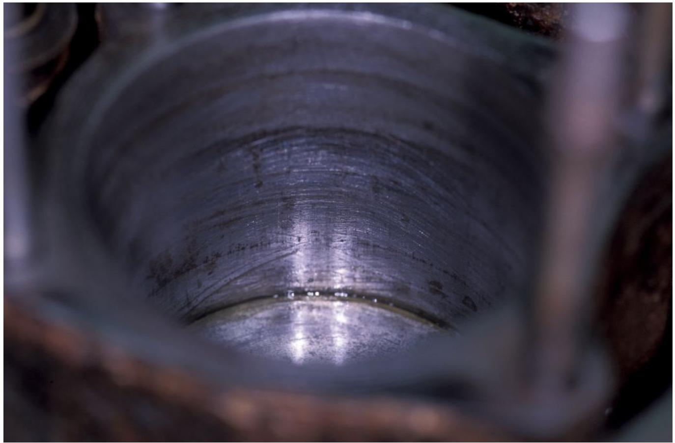
**This cylinder wall is damaged from corrosion, and as such the rings have also likely suffered as well.**
