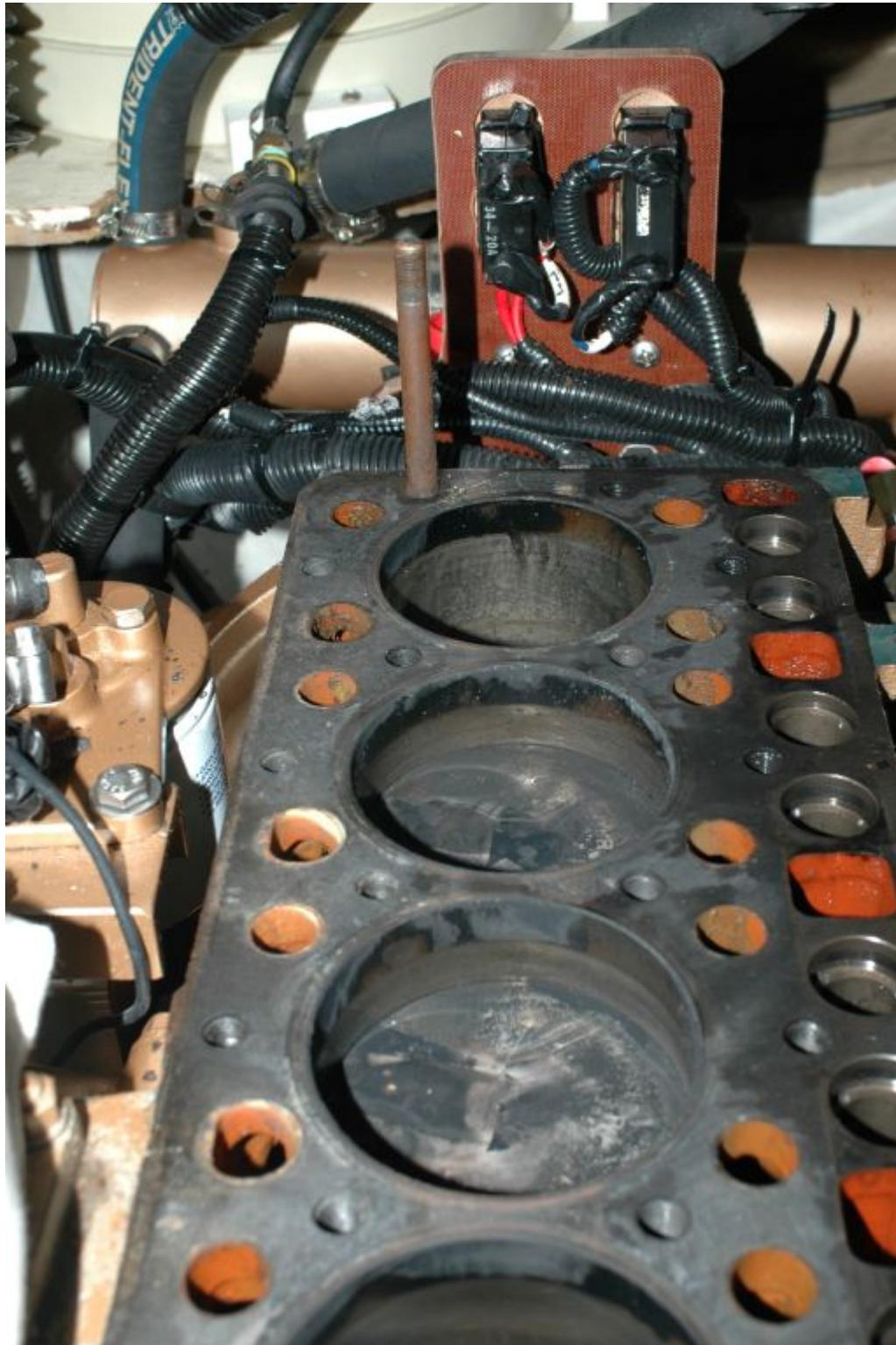
**Light loading, over-fueling, air starvation and other causes can lead to excess soot production, which in turn can cause rings to clog, and malfunction.**
