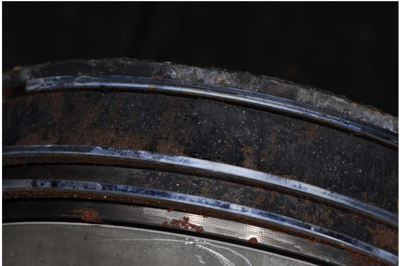
**The engine this piston was installed in suffered sea water intrusion, from a leaking aftercooler, which has caused the rings to rust.**
