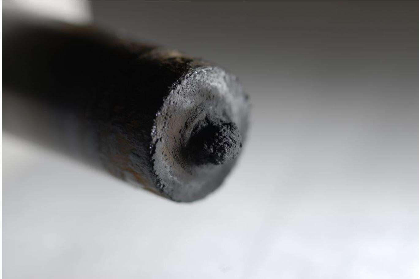
**Malfunctioning or fouled injectors can lead to excessive carbon fouling, as well as cylinder wall “washing” where fuel washes away or dilutes lubricating oil, all of which can lead to ring issues.**
