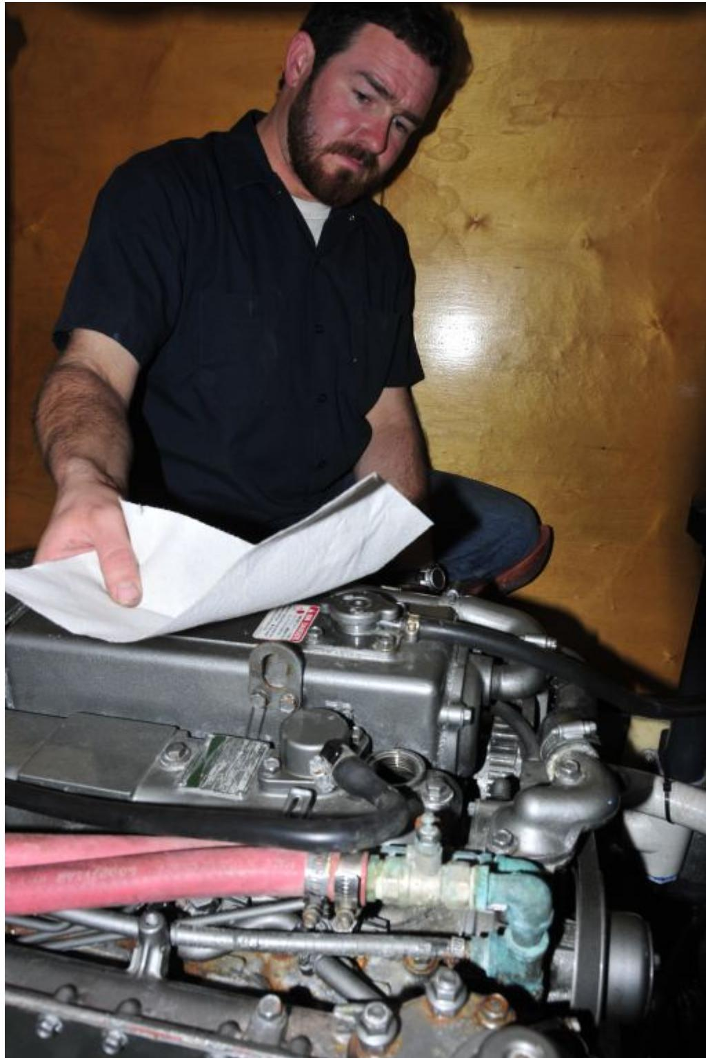
**An unofficial blow-by test.** When piston rings leak, either from soot clogging, wear, or cylinder glazing, gasses leak past or "blow-by" them into the crankcase, leading to excessive crankcase pressure.
