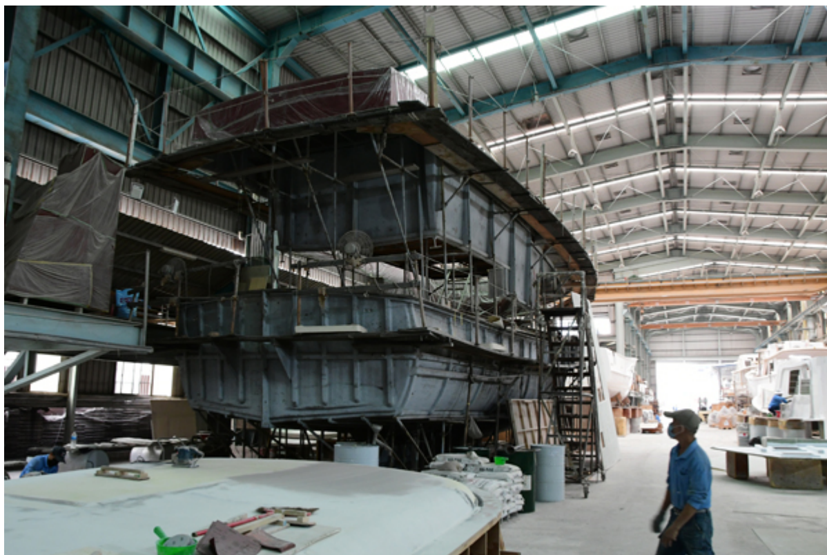
Hull and deck molds inside Asia Harbor's cavernous shed, in Kaohsiung, Taiwan.
