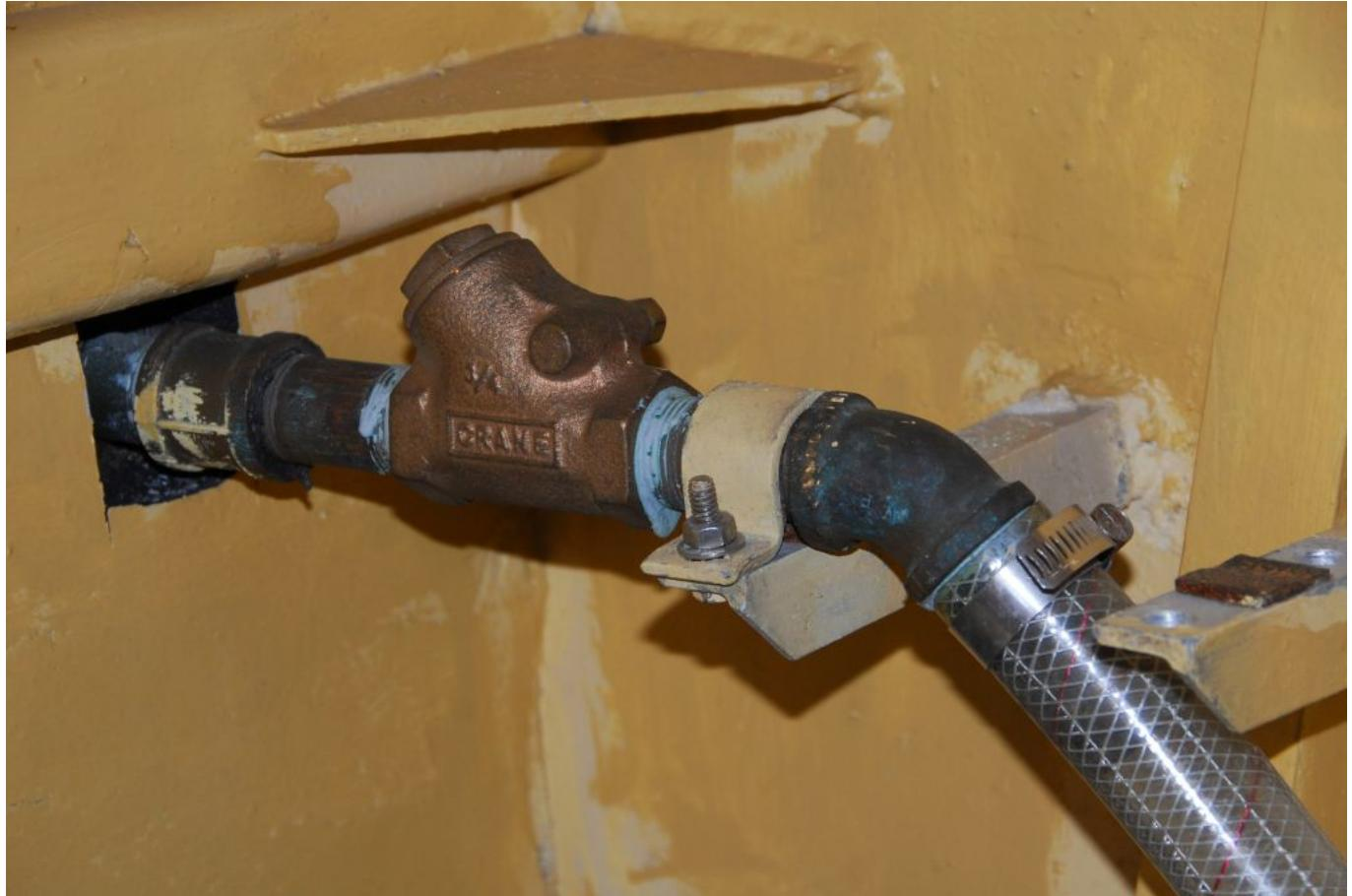
**Somewhat less objectionable, this check valve is located at the point of discharge, where at least the water column issue is eliminated, it is being used in place of an anti-siphon valve, which is a violation of ABYC Standards. A riser and antisiphon valve would accomplish the same task with less risk.**
