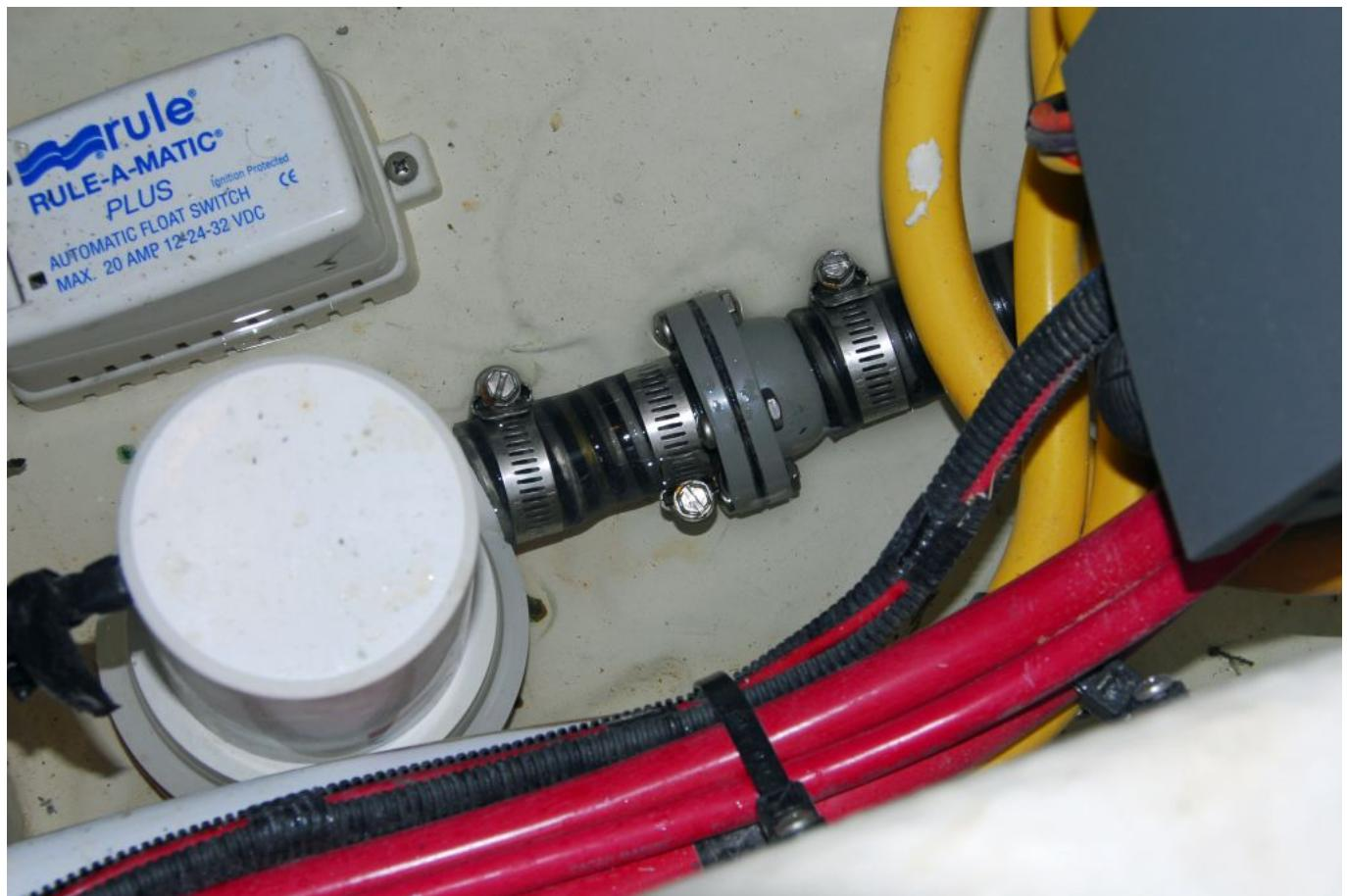
**A plastic and rubber check valve uses no metal parts other than fasteners. It's less prone to sticking and corrosion; however, like all check valves other than those that are made**
