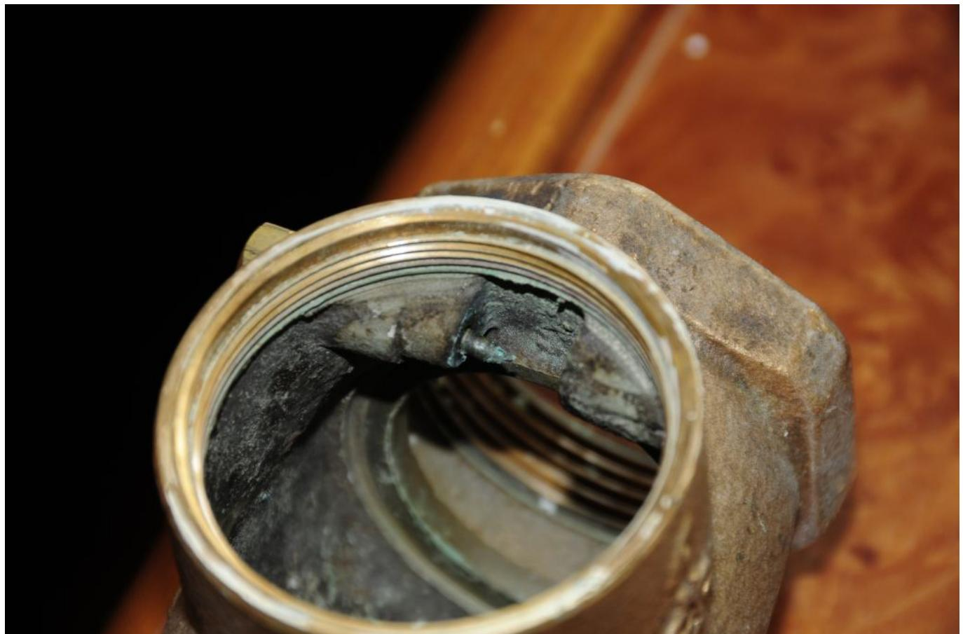
**The 'guts' of a swing check valve, used in an air conditioning system, with the gate or door removed for the photo. This one's corroded/worn out "axle" (often made from brass) allowed the gate to fall into the water stream, restricting water movement, as well as preventing it from checking flow.**
