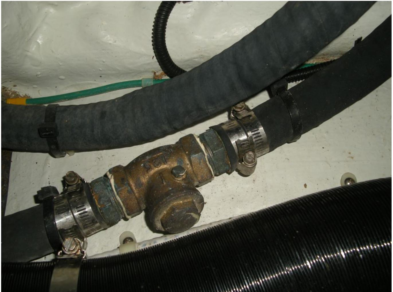
**Traditional “swing” check valves have orientation limitations. While the gate opens in the direction of intended flow, the gate should not face downward, allowing it to hang open, and the pivot point should be at or close to the 12:00 o’clock position.**
