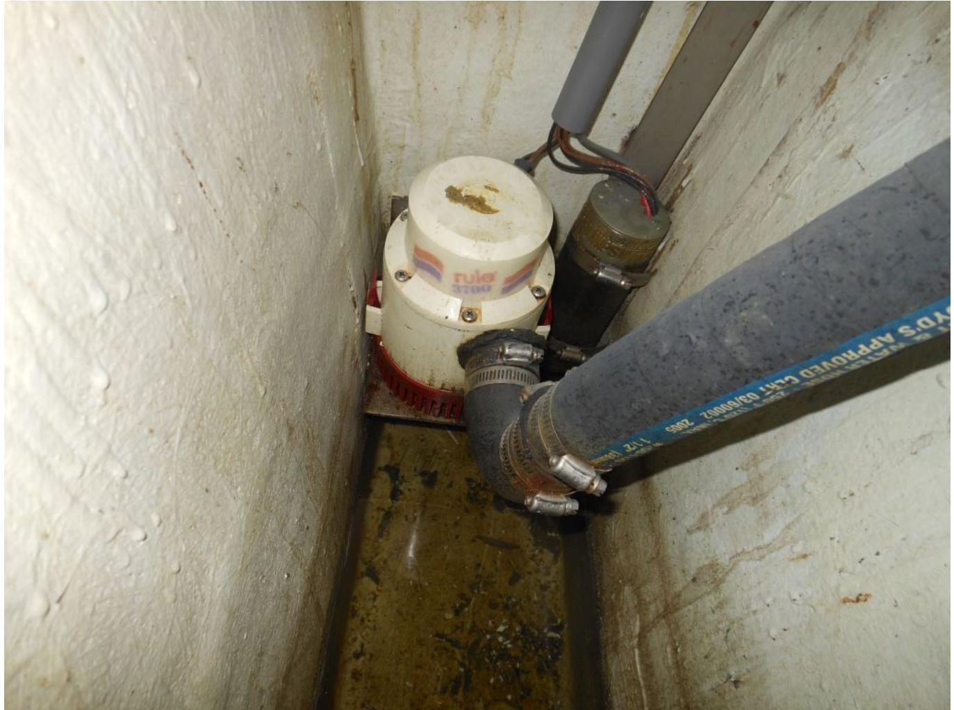
**A large-diameter hose, a deep bilge, a submersible pump, and an in-line check valve (visible in the center of the image, retained by hose clamps) can be a recipe for failure.**
