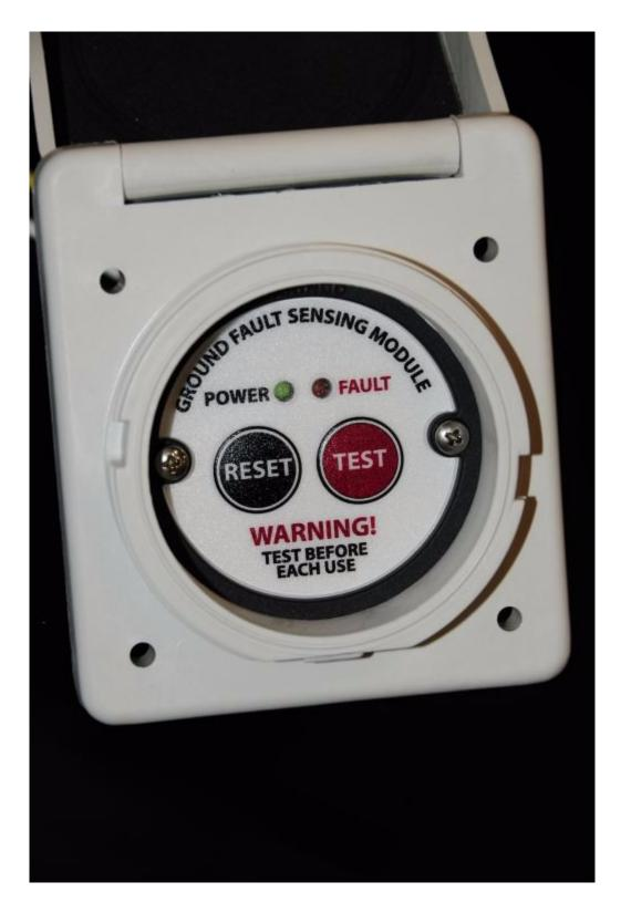
An equipment leakage circuit interrupter or ELCI, is capable of sensing faults in a vessel's AC electrical system, whereupon it will turn off power in the blink of an eye,
