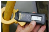
Using a sensitive leakage test device, this vessel's shore power cord is telling a potentially dangerous story.
