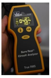
A tool such as the one shown here is capable of performing a multitude of tests on shore power installations, including proper GFCI operation, ground quality and identifying compound faults. They are not inexpensive, however, more and more boat yards are using tools like this to perform routine checks on customers' boats. I use one routinely during pre-purchase inspections and in fault analysis projects.
