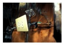
It's important to note that all receptacles, regardless of whether they are GFCI or not, must be installed within enclosures. Although this example is extreme, it's not uncommon to find even new boats where the exposed rear portion of a receptacle protrudes into a locker or other accessible space. Once again, every receptacle must be installed in a dedicated, purpose made box.
