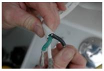
Wiring faults such as these can lead to equipment damage, short circuits or failure as well as injury to the crew. RCDs answer the call where equipment protection is concerned, however, although not specifically designed for it they may also prevent electrocutions.
