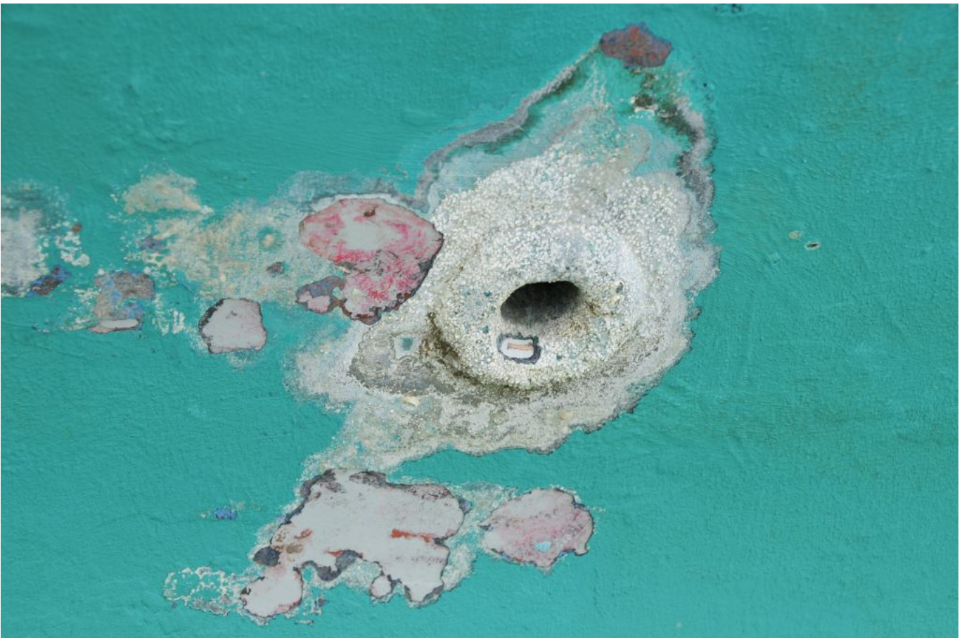
Two textbook examples of cathodic disbondment, a phenomenon
