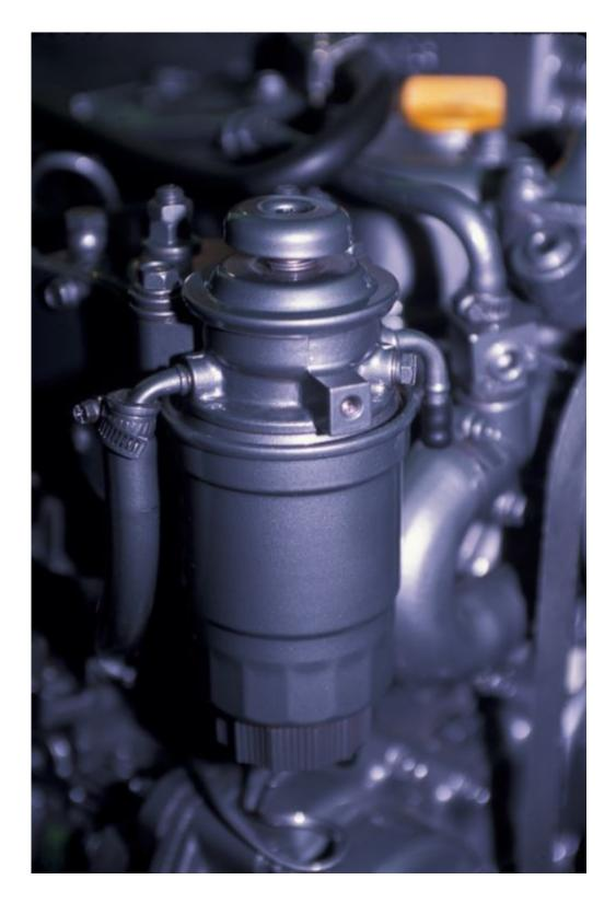
A clogged secondary fuel filter will cause an engine to starve for fuel, and shut down, without necessarily registering anything unusual on the primary filter's vacuum gauge.
