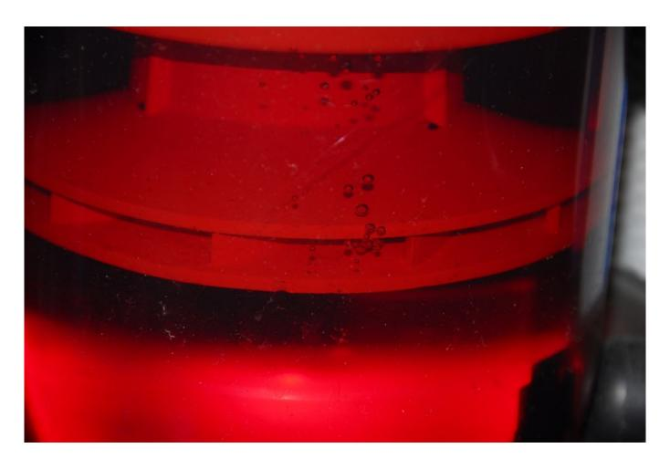
Air leaking into the fuel system upstream of the primary filter, will accumulate here, and eventually make its way to the engine's high pressure pump, which in turn will lead to a shut down.
