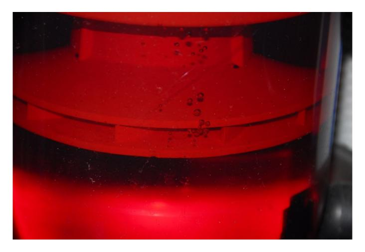
Air leaking into the fuel system upstream of the primary filter, will accumulate here, and eventually make its way to the engine's high pressure pump, which in turn will lead to a shut down. Last month I reviewed some of the reasons an engine or genset might not start. I confined that discussion mainly to electrical gremlins, wherein the engine will not crank. In this month's column I'll delve into reasons an engine might crank but not actually start.
