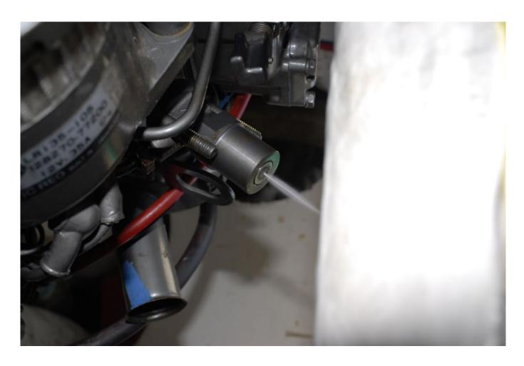
A properly functioning injector will develop a uniform spray pattern, one that atomizes fuel into a mist, like the one shown here.
