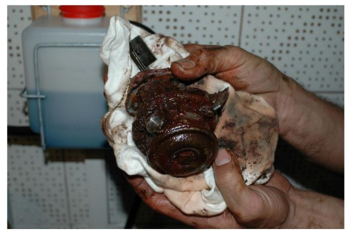
Fuel lift pumps are simple and robust, however, they do wear out, and many include integral filters or screens, which can become clogged.
