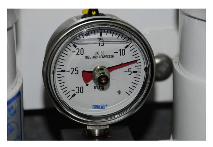
The primary fuel filter vacuum gauge is an invaluable ally in failure to start troubleshooting scenarios.
