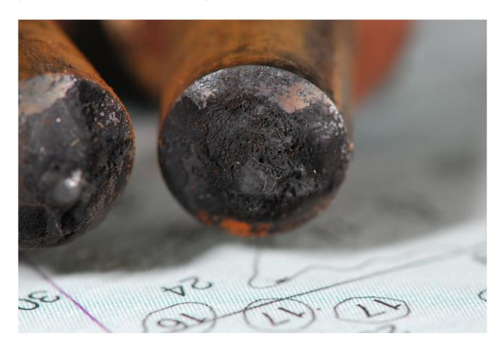
Fouled or otherwise malfunctioning injectors can make an engine difficult to start.
