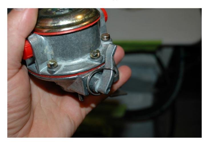
The manual lever on a fuel lift pump is used to prime, and bleed air from, the fuel system.
