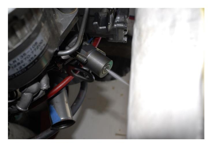
A properly functioning injector will develop a uniform spray pattern, one that atomizes fuel into a mist, like the one shown here.
