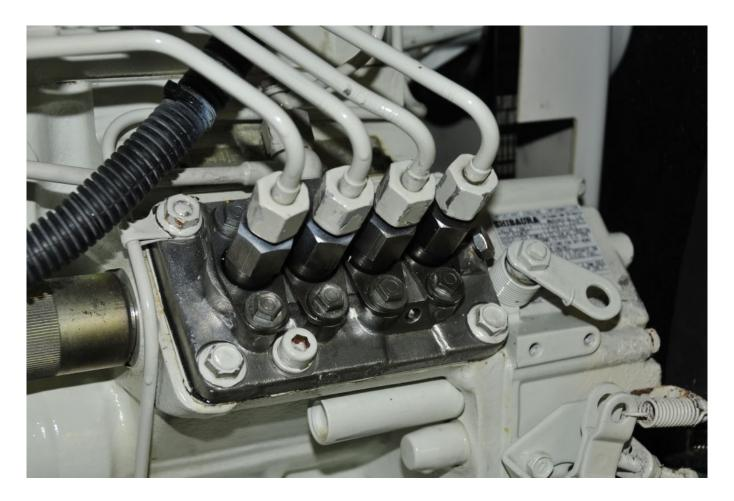
Injection pumps can fail, however, this is relatively rare. Dirt and water, on the other hand, can quickly bring even the most robust injection pump to its knees.
