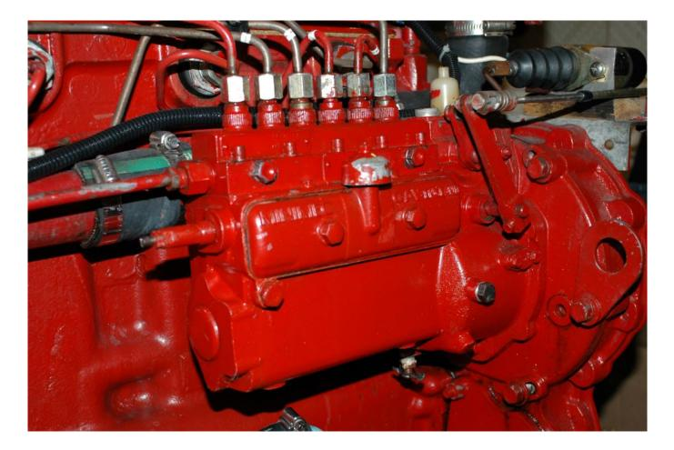
Most conventional high pressure injection pumps use some type of electro-mechanical mechanism to allow fuel to flow, or stop flowing, that is used to stop the engine. If it malfunctions, the engine may not start (or it may not stop). The pump seen here uses a solenoid plunger, visible with the rubber bellows, in the upper right, that is engaged to stop fuel flow for shut down purposes.
