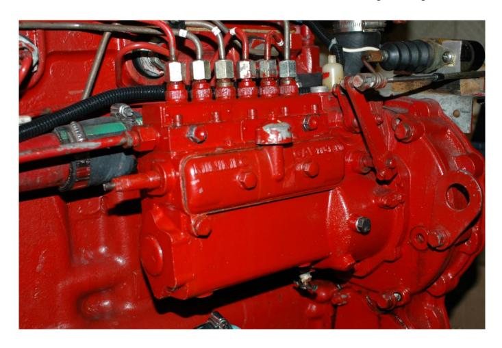
Most conventional high pressure injection pumps use some type of electro-mechanical mechanism to allow fuel to flow, or stop flowing, that is used to stop the engine. If it malfunctions, the engine may not start (or it may not stop). The pump seen here uses a solenoid plunger, visible with the rubber bellows, in the upper right, that is engaged to stop fuel flow for shut down purposes.
