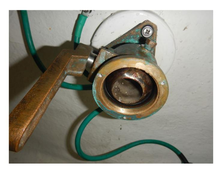
This image, of a partially disassembled seacock, illustrates why it is necessary to ensure that the valve is open when applying grease using the zerk fitting; the grease will fill the void between the ball and the inside of the seacock body. If the valve were closed, grease would be pumped into the ball's void, where it would do no good.
