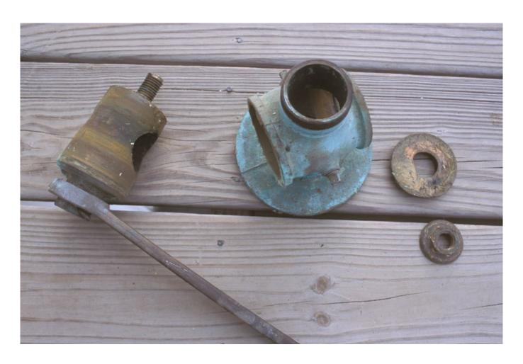
Cone-style seacocks can be disassembled, cleaned, lapped using valve grinding compound, greased and reassembled. One of the drain plugs on the one shown here could have a zerk fitting installed.
