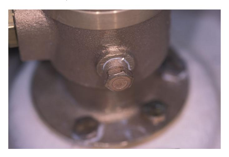
Drain plugs used on metallic seacocks must be made from bronze and not brass. Bronze plugs in the size typically used, 1/8"
