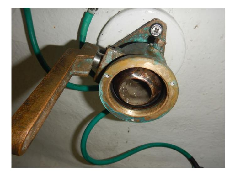
This image, of a partially disassembled seacock, illustrates why it is necessary to ensure that the valve is open when applying grease using the zerk fitting; the grease will fill the void between the ball and the inside of the seacock body. If the valve were closed, grease would be pumped into the ball's void, where it would do no good.
