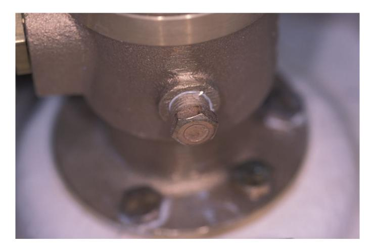
Drain plugs used on metallic seacocks must be made from bronze and not brass. Bronze plugs in the size typically used, 1/8" - 27 NPT, are not commonly available, which means it may be necessary to source them from the seacock manufacturer.
