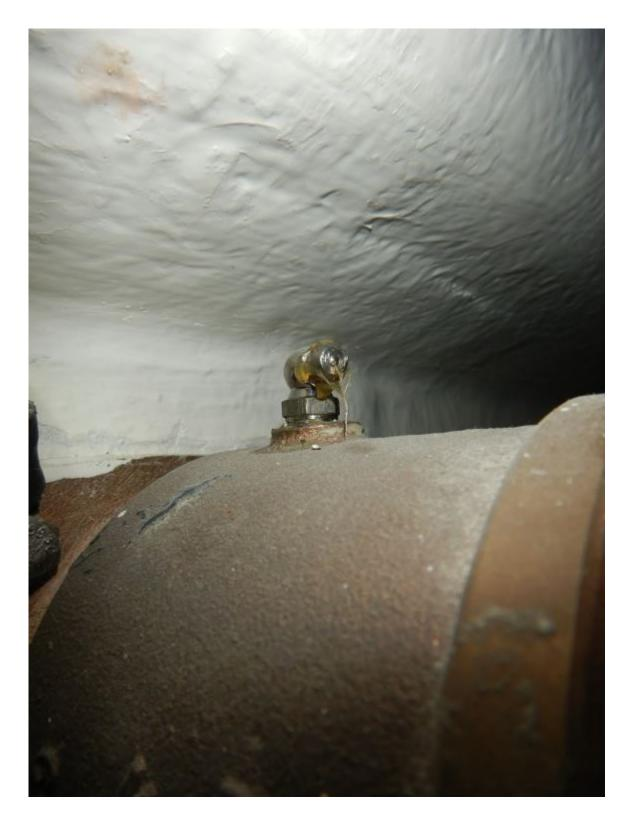
The addition of zerk fittings has been a boon to seacock maintenance, making it easy to keep them lubricated and functional. It's important that zerk fittings remain accessible after a seacock has been installed. In this case, a 90 degree fitting has been used to ensure a grease gun can be attached.
