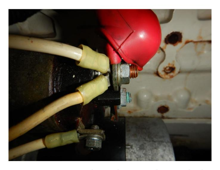
ABYC Standards call for ring terminals to be installed in size order, from largest to smallest; the example shown here is incorrect. Getting this wrong can lead to high resistance, and the associated issues that accompany it.
