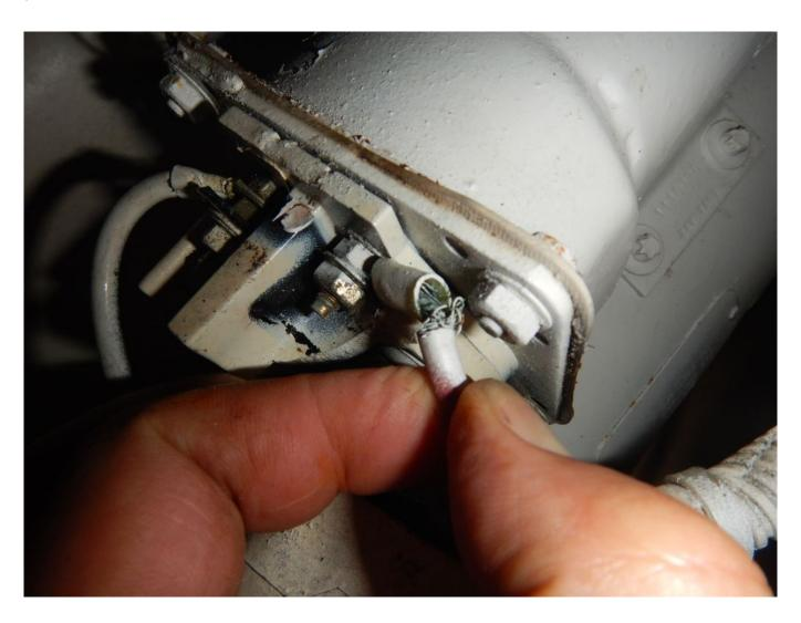
Poor connections account for a significant portion of failure to crank scenarios.
