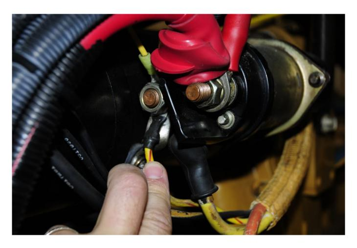
The wire that sends voltage from the key switch to the starter solenoid is typically yellow with a red stripe. If, when holding the key in the crank position, no voltage is measured on this wire at the starter solenoid, then the starter will not engage.
