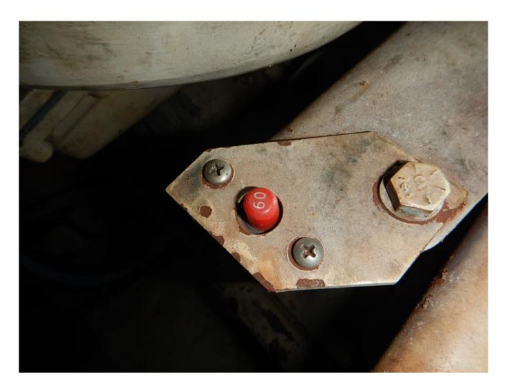
Circuit breakers and fuses at the engine that supply power to the instrument panel, and key switch, are a critical link in the starting process. If they are tripped or blown, the instrument panel, and key switch, will be dead.
