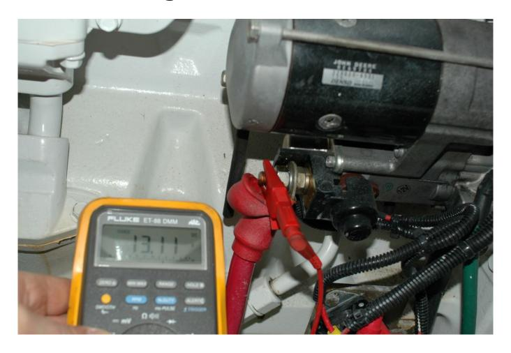
Voltage at the starter's primary post should be nearly the same as that measured at the battery, if the difference is significant, then a connection issue exists.
