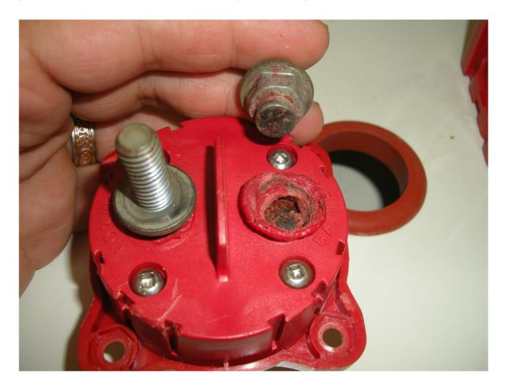
A failed battery switch can account for a no crank issue, these should be carefully checked, including tugging on the study and ring terminals to ensure they are tight.
