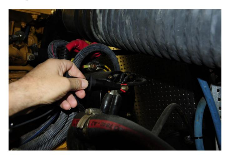
When taking voltage measurements at the engine, be sure to connect your multimeter test lead to the same DC negative source used by the engine.
