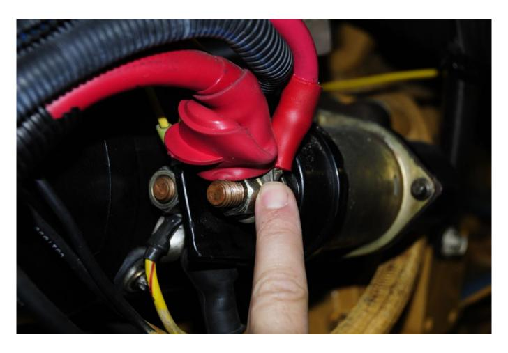
The large positive post on the starter should have voltage available to it when ever the battery switch is on.
